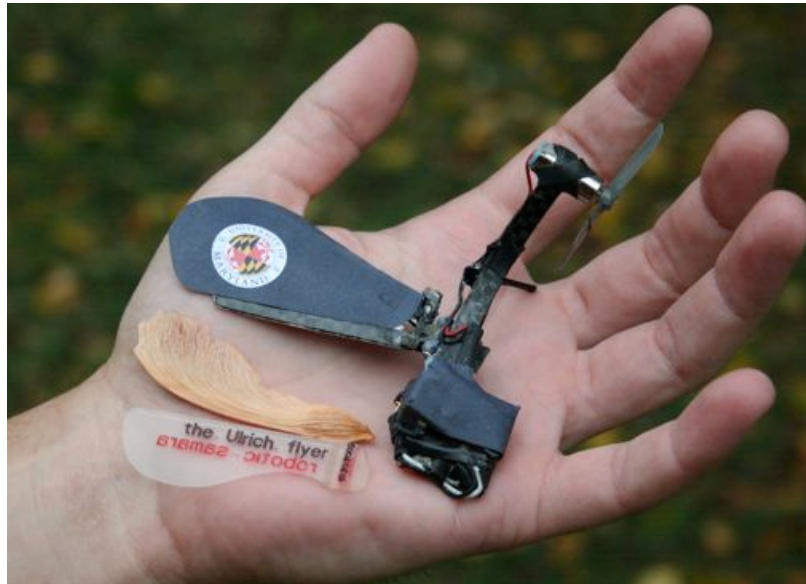
Figure 3.17: Smallest robotic samara constructed.
