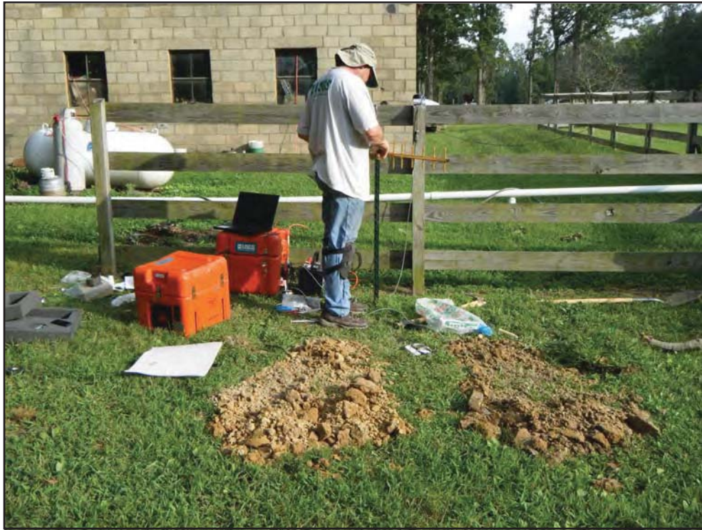
Figure 3-2. Temporary seismic station in epicentral region of the Mineral earthquake Steve Ploetz, a field engineer, installs a temporary USGS seismic station named PTRD in Spotsylvania County, Virginia, one of over 30 installed by a variety of organizations within three days after the mainshock. Photo taken thanks to Alana Leeds who agreed to meet with me during the days immediately following the mainshock in the epicentral region near the town of Mineral, VA.
