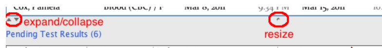
Figure D.9: The split pane between the tables permit users to modify default table sizes. While the upward/downward arrows (leftmost) are to expand/collapse, dragging the dot (middle) resizes.
