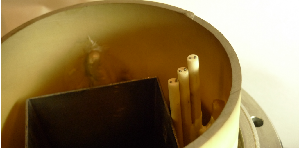
Figure 4.7 – The alumina limiter is shown surrounding the X-band horn and langmuir double probes.
