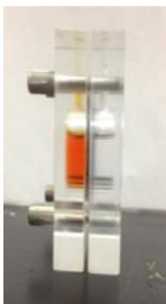
Figure 4: Nafion Leakage Test Initial setup: Left chamber contains 3 mL aqueous bromothymol blue (0.01% concentration). Right chamber contains 3 mL deionized water.
