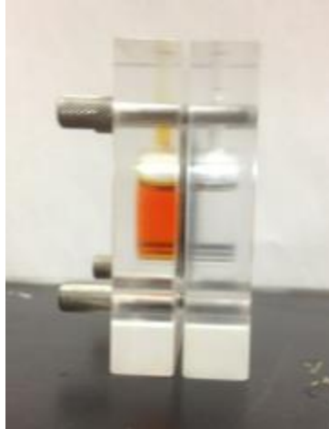
Figure 2: Nafion Initial setup: Left chamber contains 3 mL aqueous bromothymol blue (0.01% concentration). Right chamber contains 3 mL deionized water.
