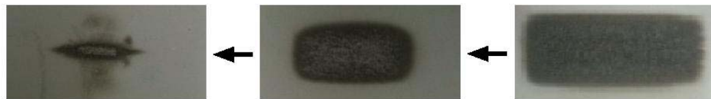
Beam profile at various locations of the PLD system without an optical diaphragm: @ target @ view port @ focusing lens
