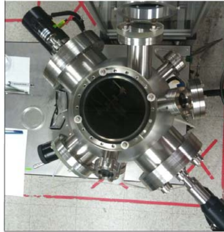
Figure 1. PLD deposition chamber. Left is the schematic of the chamber showing various parts: 1 is the incident laser beam, 2 is the optics, 3 is the laser port, 4s are the glass view ports, 5 is the controlled target holder, 6 is the controlled sample holder, and 7 is the ejected plume from the PLD target. Right is the top view of the actual growth chamber.
