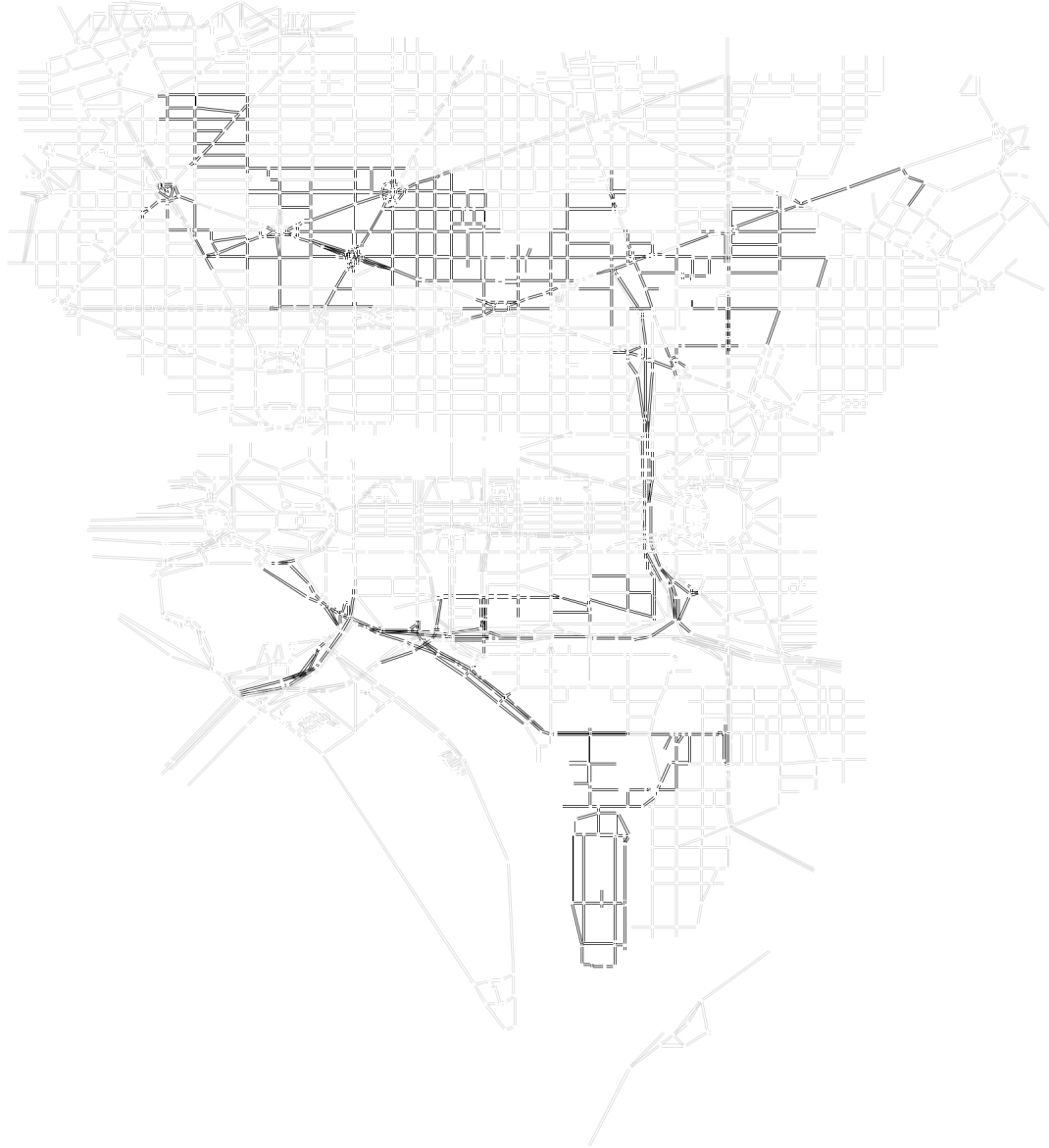
Figure 2.9: Portion of the Washington, DC street network before the initialization procedure is applied
