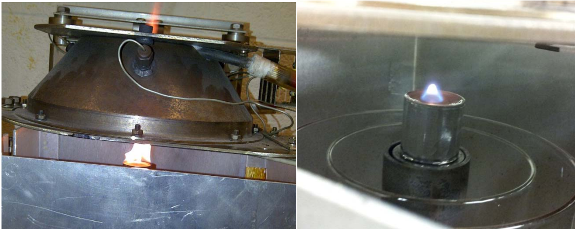
Figure 29: PMMA Fuel Flame Size Before (Left) and After (Right) Exposure to Clean Agent
