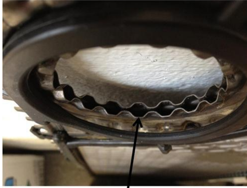
Refrigerant Flow Channel
