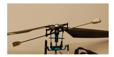
Figure 1.3: Flybars are used to mechanically stabilize helicopters.
