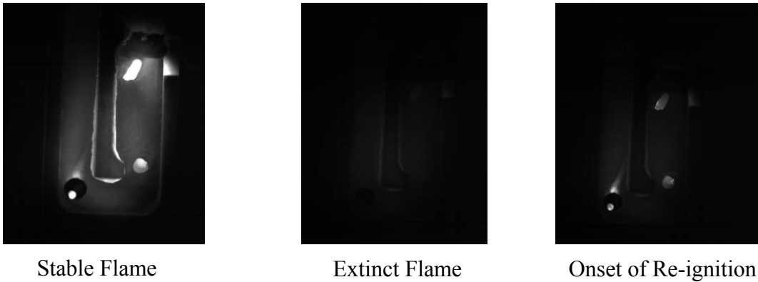
Figure 4.20. High speed images of an FREI event. From left to right: Stable flame, extinct flame, onset of re-ignition
