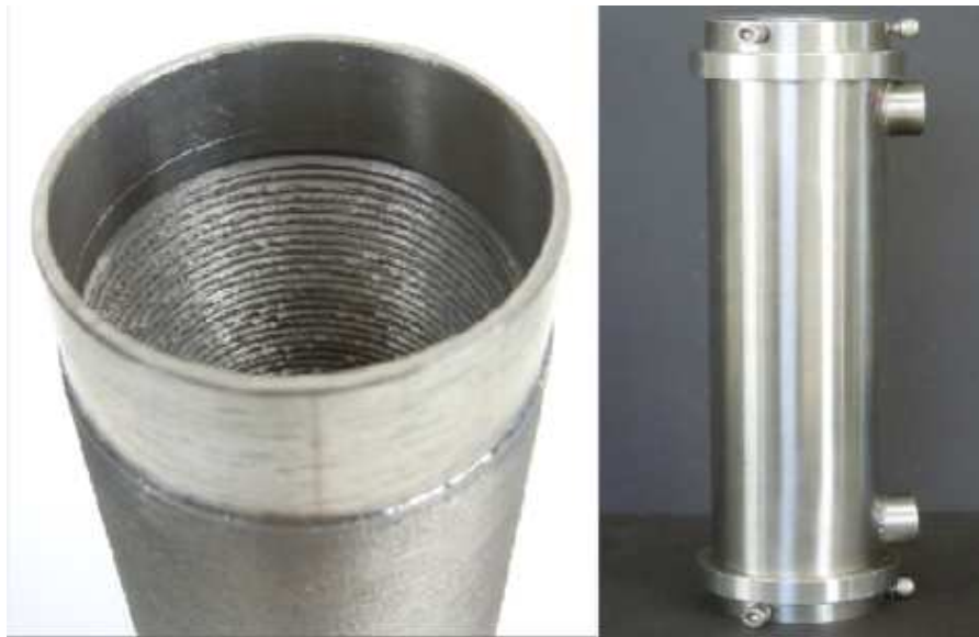
Figure 5-7: Nickel microgroove tube and HX assembly
