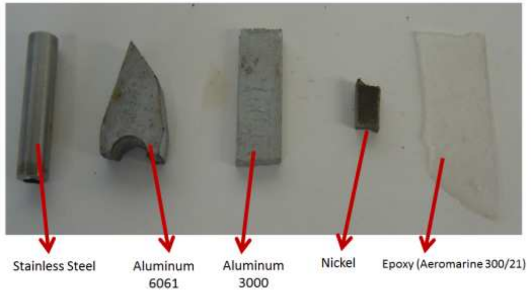
Figure 6-35: Samples of heat exchanger materials before water-ammonia solution compatibility testing
