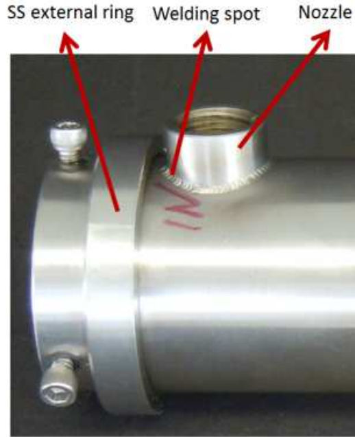
Figure 5-6: SS tube welding assembly
