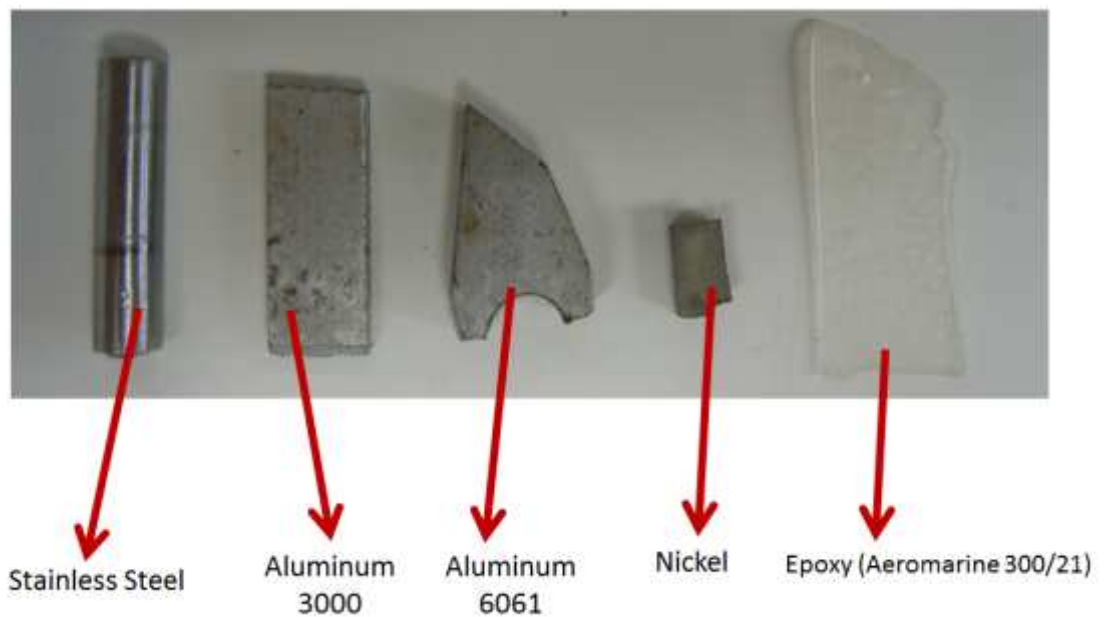
Figure 6-36: Same materials after submerging in the ammonia –water solution for 4 months
