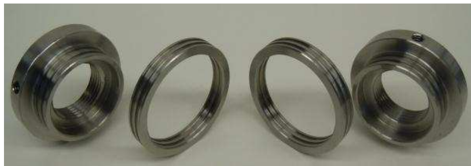
Figure 5-8: Steel flanges used in the assembly
