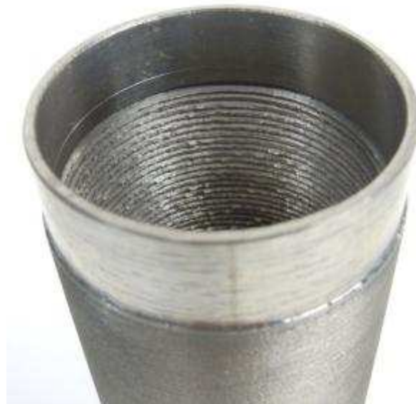
Figure 6-37: Nickel high aspect ratio microgroove tube
