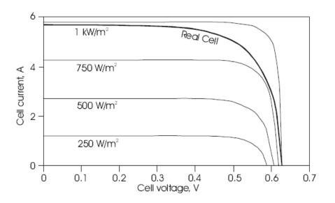
Figure 7: I-V characteristics of PV cells under different irradiance levels (Roger and Ventre, 2005)
