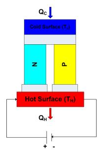
Figure 14: Schematic of a single thermoelectric device
