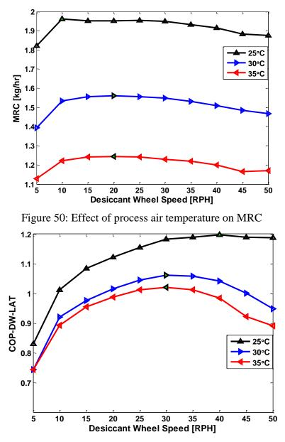
Figure 51: Effect of process air temperature on COP<sub>Lat</sub>
