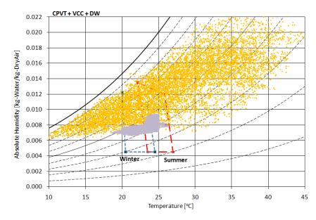
Figure 39: The hourly ambient conditions for Abu Dhabi and indoor space conditions for one year simulation (CPVT+VCC+DW).
