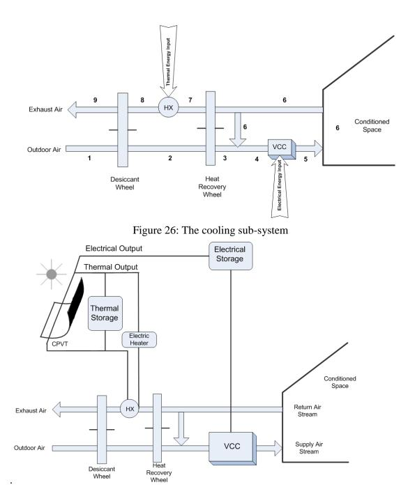
Figure 27: Schematic of the hybrid solar cooling system.
