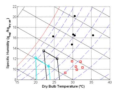
Figure 68: Inlet (Black Circles) and outlet conditions (Red Squares) of the desiccant wheel cycle
