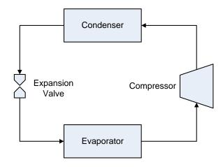
Figure 13: Schematic of a VCC
