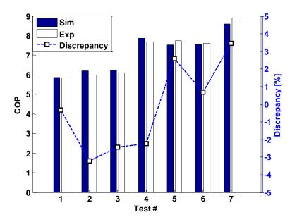
Figure 89: The experimental VCC coefficient of performance
