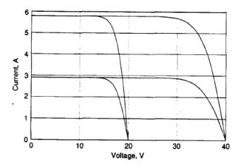
Figure 9: I-V curves of PV cells connected various series and parallel arrangements (Duffie and Beckman, 1991)
