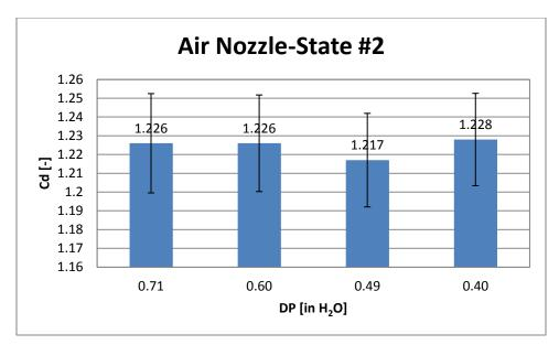
Figure A-6: Nozzle discharge coefficient at state 2 vs. nozzle's pressure drop
