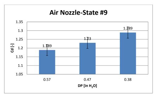
Figure A-8: Nozzle discharge coefficient at state 9 vs. nozzle's pressure drop
