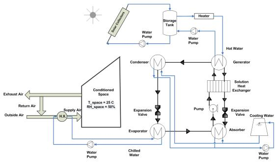
Figure B-1: Solar Powered Absorption Cycle
