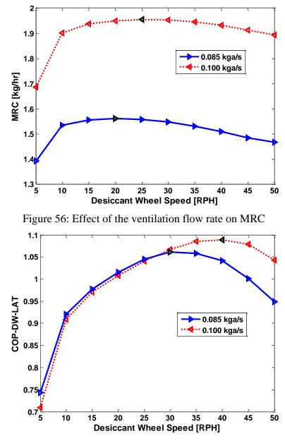
Figure 57: Effect of the ventilation flow rate on COP<sub>Lat</sub>
