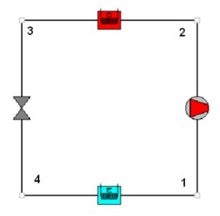
Figure 85: Vapor compression cycle in VapCyc
