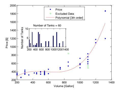
Figure D-1: The cost of different hot water storage tanks
