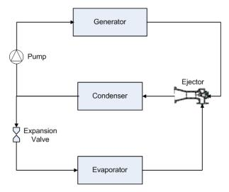
Figure 21: Steam Ejector Cycle
