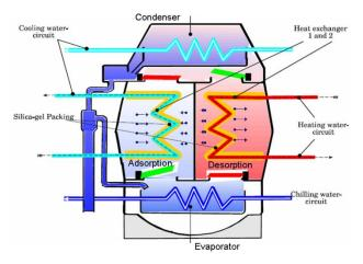
Figure 20: Adsorption cycle (GBU, 1995)
