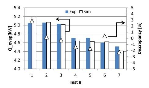
Figure 81: Evaporator capacity
