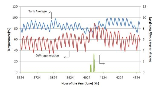
Figure 30: Simulated performance of the DW for the month of June The performance of the cooling sub-system is simulated at  $T_{amb} = 45^{\circ}$ C and  $w_{amb} = 15$  gw/kga. Figure 31 shows the psychrometric processes with state points corresponding to
