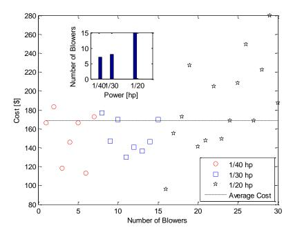
Figure D-2: The cost of air blowers.
