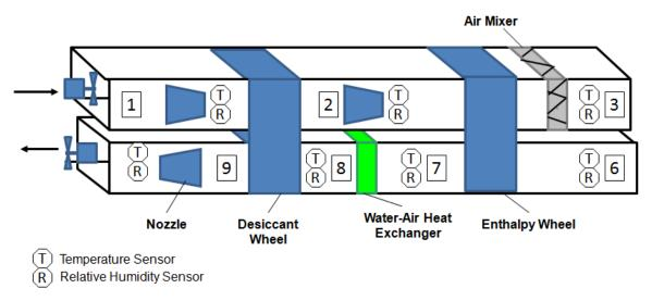
Figure 42: Experimental setup
