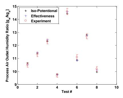
Figure 75: Desiccant wheel process outlet humidity ratio
