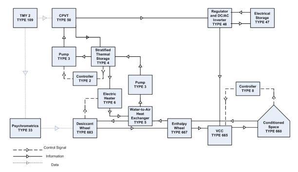
Figure 28: System information flow diagram.
