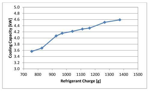
Figure C-2: Cooling capacity as a function of refrigerant charge
