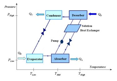
Figure 19: Diagram of an absorption cycle
