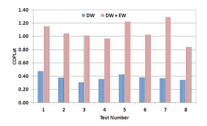
Figure 62: COP<sub>Lat</sub> with and without the enthalpy wheel
