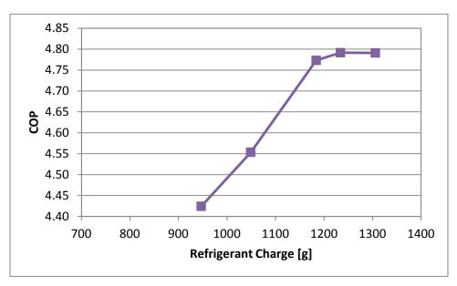
Figure C-3: COP as a function of refrigerant charge
