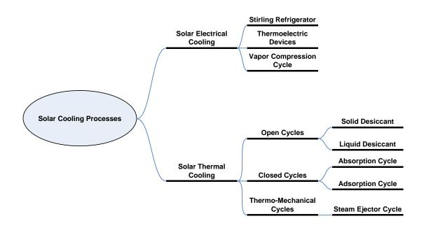
Figure 12: Solar cooling processes classifications
