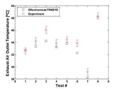
Figure 78: Enthalpy wheel exhaust outlet temperature
