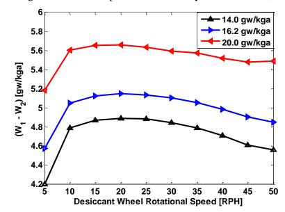
Figure 54: Effect of process air humidity ratio on process air humidity difference
