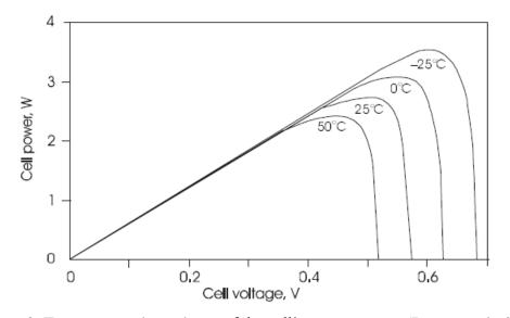
Figure 8: Temperature dependence of the cell's power output (Royne et al., 2005)
