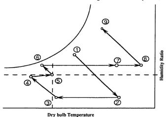
Figure 17: Pennington cycle for cooling and dehumidification
