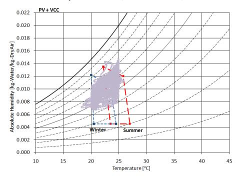
Figure 40: The hourly space conditions for one year simulation (PV + VCC)
