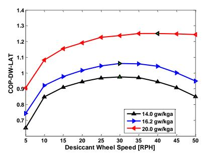
Figure 53: Effect of process air humidity ratio on COP<sub>Lat</sub>
