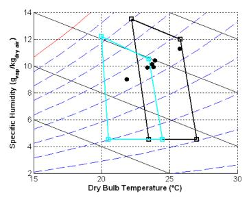
Figure 69: Indoor conditions for the hybrid A/C at various operating conditions Moreover, the VCC can be operated differently when coupled with a DWC. Since the DWC accommodates the latent load, the VCC has to accommodate the sensible load
