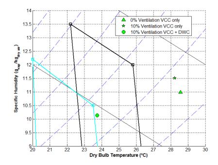
Figure 66: Indoor conditions for the hybrid A/C and the standalone VCC
