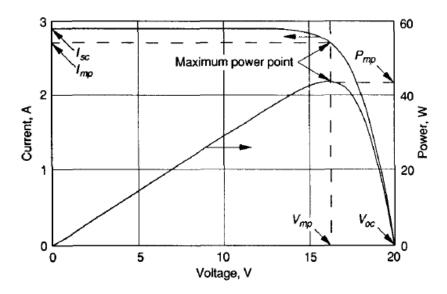
Figure 5: Typical I-V and power characteristics of a PV module (Duffie and Beckman, 1991)
