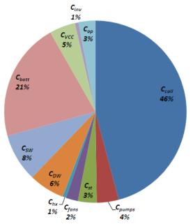
Figure 96: The hybrid A/C cost breakdown
