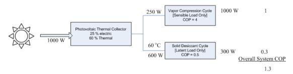
Figure 24: COP of the proposed hybrid solar air conditioner
