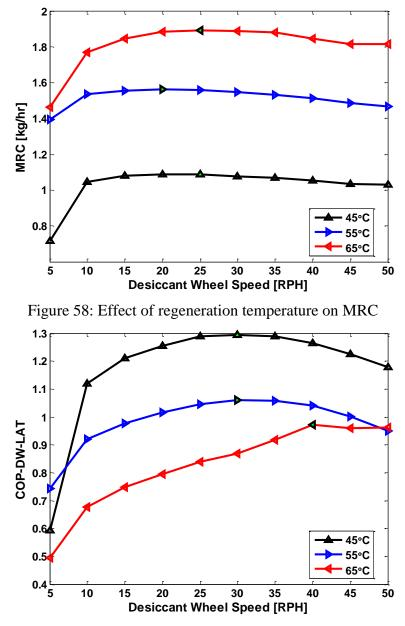
Figure 59: Effect of regeneration temperature on COP<sub>Lat</sub>
