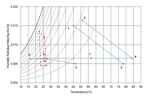
Figure 31: Air state points in various locations in the cooling sub-system.
