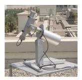
Figure 4: Pyranometer and Pyrheliometer
