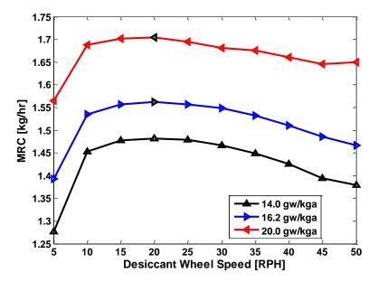
Figure 52: Effect of process air humidity ratio on MRC
