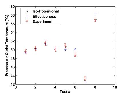
Figure 74: Desiccant wheel process outlet temperature
