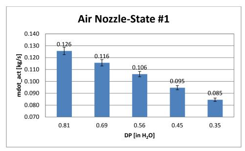
Figure A-1: Actual mass flow rate at state 1 vs. nozzle's pressure drop
