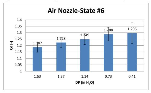
Figure A-7: Nozzle discharge coefficient at state 6 vs. nozzle's pressure drop
