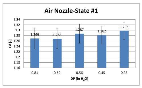
Figure A-5: Nozzle discharge coefficient at state 1 vs. nozzle's pressure drop
