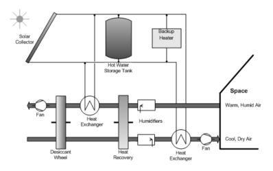
Figure 16: Schematic of a desiccant cooling ventilation cycle (Henning, 2007b)
