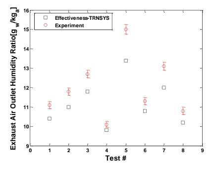
Figure 79: Enthalpy wheel exhaust outlet humidity ratio
