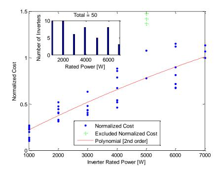
Figure D-3: The normalized cost of different inverters.
