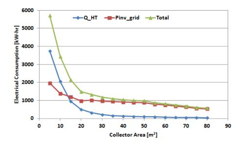
Figure 35: The effect of the collector area on the external energy needed
