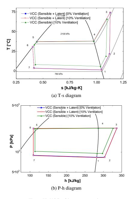
Figure 70: VCC refrigerant state points
