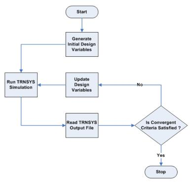
Figure 71: MATLAB optimization flow diagram
