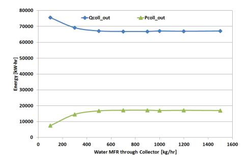
Figure 32: The effect of the collector MFR on its outputs.
