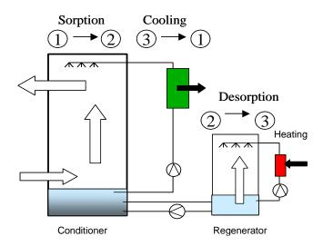
Figure 18: Schematic of a liquid desiccant system
