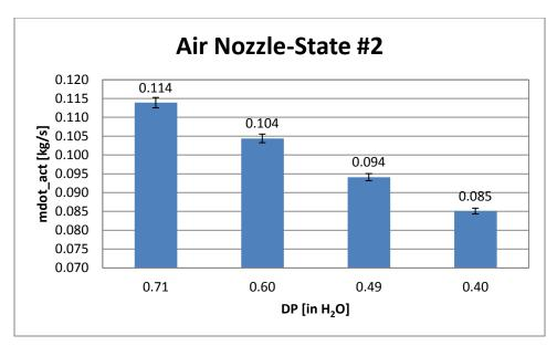
Figure A-2: Actual mass flow rate at state 2 vs. nozzle's pressure drop
