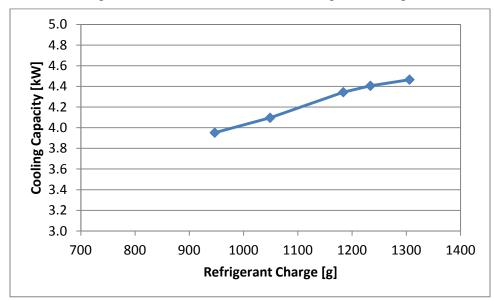
Figure C-4: Cooling capacity as a function of refrigerant charge
