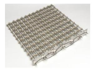
Figure 65: Electric air heater to represent the space sensible load.
