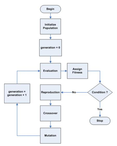
Figure 72: A flowchart of GA's working principle (Deb, 2001)
