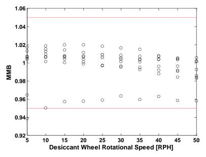
Figure 48: Moisture Mass Balances of all the tests
