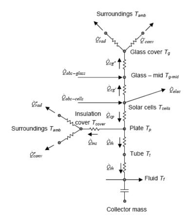
Figure 73: Thermal network of the CPVT collector (Coventry, 2005)
