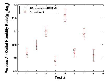
Figure 77: Enthalpy wheel process outlet humidity ratio
