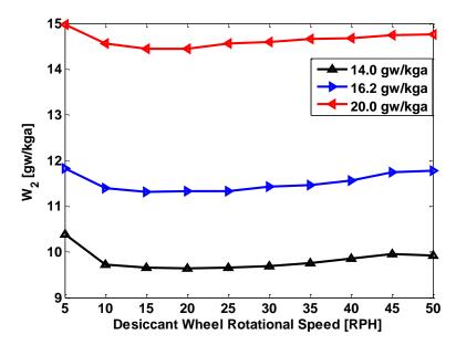
Figure 55: Effect of process air humidity ratio on DW's process outlet humidity ratio Investigating the effect of increasing the ventilation mass flow rate was possible due to utilizing variable speed fans. Figure 56 shows that as the mass flow rate across the DW is increased, the MRC value increases. In order to maintain the same regeneration temperature, more heat is required for the higher mass flow rate. Therefore, the  $COP_{Lat}$ for the higher mass flow rate reduces as shown in Figure 57.
