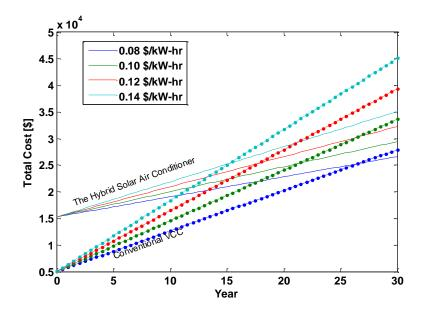
Figure 95: Total cost of the proposed system vs. conventional VCC
