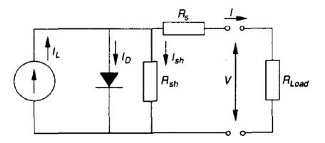
Figure 6: Equivalent circuit of a PV cell (Duffie and Beckman, 1991)
