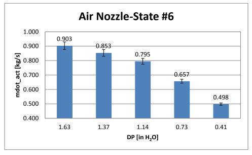
Figure A-3: Actual mass flow rate at state 6 vs. nozzle's pressure drop
