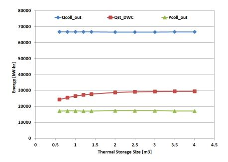
Figure 33: Thermal storage size vs. energy delivered.
