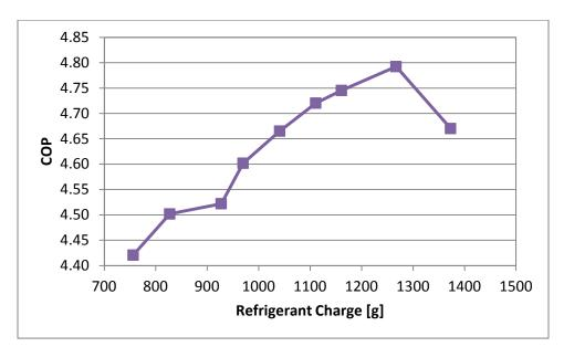
Figure C-1: COP as a function of refrigerant charge
