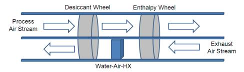
Figure 41: Desiccant wheel cycle schematic
