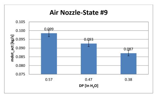
Figure A-4: Actual mass flow rate at state 9 vs. nozzle's pressure drop The corresponding Nozzle discharge coefficients are shown in Figures A-5 to A-8, respectively.
