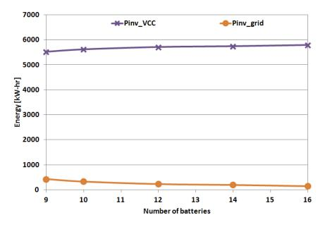
Figure 34: Effect of the electrical storage size on the electrical energy delivered. One of the key parameters of any solar cooling system that highly affects its performance and initial cost is the collector area. The effect of the CPVT collector area on the amount of external electrical energy needed is shown in Figure 35. The results show that as the
