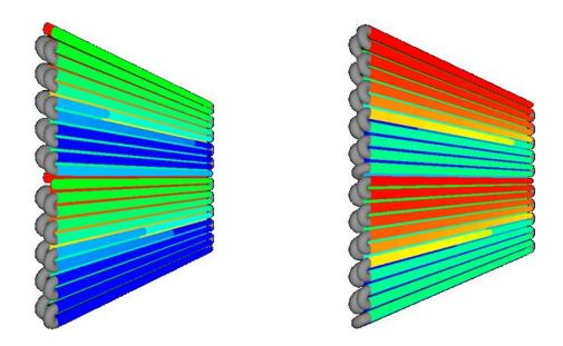
Figure 80: Evaporator circuitry and temperature distribution in CoilDesigner
