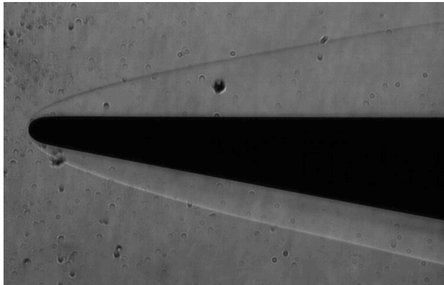
Figure 5.2. Plus 5 degrees AOA. The shock on the bottom is darker in spots and less straight, indicating shock unsteadiness. The boundary layer is also significant.
