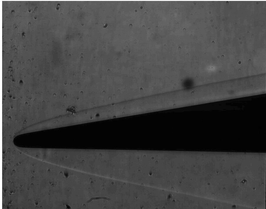
Figure 5.1. Minus 5 degrees AOA. The top has a more developed boundary layer and is unsteady. The shock is not as straight and some of the darker regions compared to Figure 5.2 correspond to places where the shock wobbles slightly.
