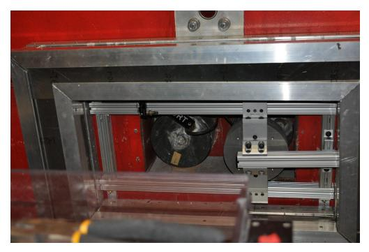
Figure 8-9: Image of the collar installed on the reactor face. Its design still allows for movement of the shutter.
