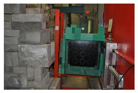
Figure 8-13: This image shows the north side of the cave installed against the reactor face.
