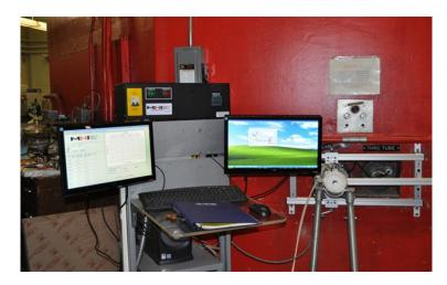
Figure 8-26: MHI robust radiator<sup>™</sup> connected to the control system with DACS software system open.
