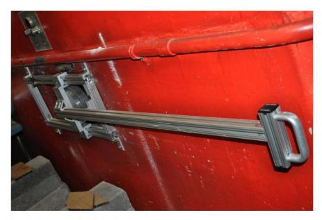
Figure 5. Handle controlling shutter for beam port.
