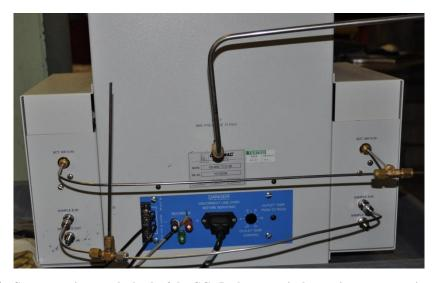
Figure 8-24: Gas connections on the back of the GC. In the center is the carrier gas connection (He). The upper connections on the left and right are for operating the pneumatically actuated sample valves. Below those are the sample inlets.
