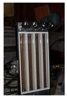
Figure 8-15: This image shows the regulator system used to deliver the research grade He to the samples and to the GC, as the carrier gas.
