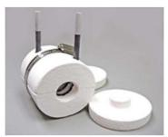
**Figure 4.** Photo of heater being used in experiment. The heater is 4 inches wide with a 1 in opening. This heater contains no parts that will become Co-60 upon irradiation. Heater will be treated as RAM after experiments.
