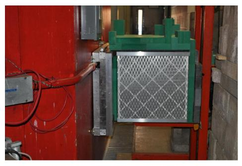
Figure 8-12: This image shows the south filtered side of the cave in place against the reactor face.
