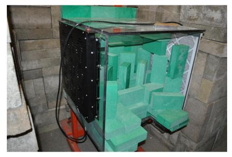
Figure 8-11: View of the interior of the cave. This photograph shows the random arrangement of the borated polyethylene blocks inside the cave, as well as the fans and filter on either side of the cave.
