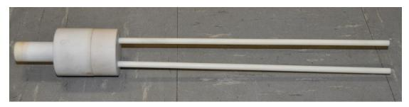
Figure 8-20: Photo of sample chamber used for east beam port experiments.
