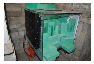
**Figure 9.** Cave built for shielding of east reactor building wall and also for cooling of heater. This is a 24in by 24-in Lexan box. Fans exhaust toward rear exit door and provide 945 cfm for cooling of the heater. Filled with 3 complete layers of borated poly bricks plus arrangement of bricks to ensure adequate air flow
