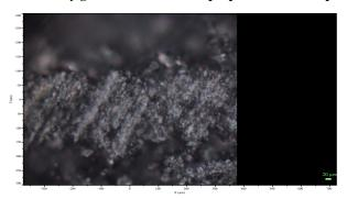
Figure B-93: Image of 2020 AG 45 MGy gamma irradiated sample prior to Raman spectra collection.
