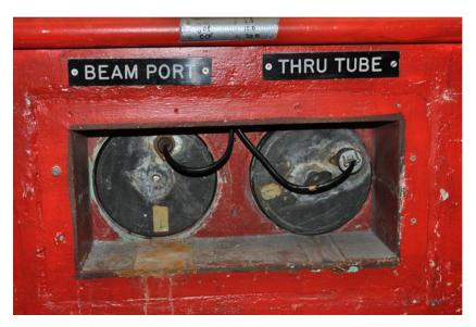
Figure 7-6: Outside of East Beam Port with the normal plugs installed.
