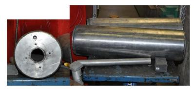
**Figure 3.** Head-on view and length-wise view of the modified beam plugs, which will be inserted into East Beam Port for experiments. There are two modified beam plugs, 31-in long Al-clad, concrete-filled plugs. They have a 2-in hole in the center to allow radiation out from the core.
