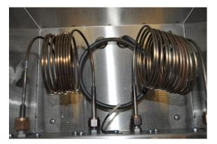
Figure 8-23: Installed columns in the Gow-Mac 400.
