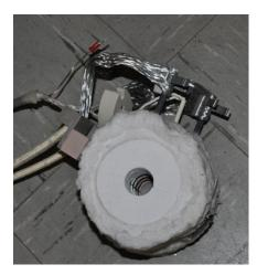
Figure 8-25: MHI robust radiator<sup>™</sup> used for east beam port experiments.
