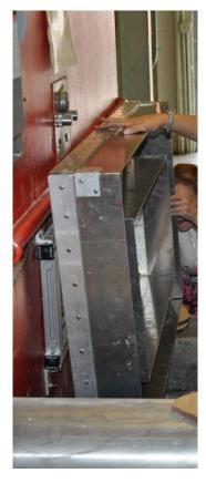
Figure 8-8: Fitting of the collar onto the face of the reactor.
