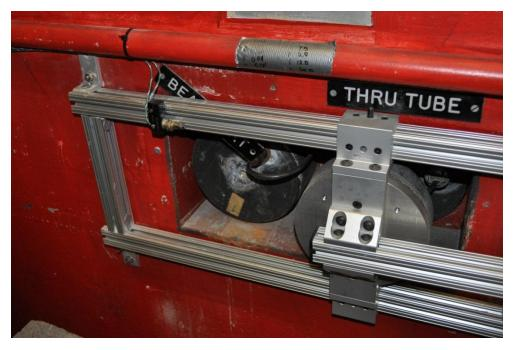
Figure 8-4: Close-up view of shutter system. This view shows how the shutter may be used for both the beam port and the through tube.
