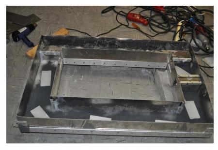
Figure 6. Photograph of the inside of the collar to be mounted on face of east reactor during filling with wax and boron carbide mixture
