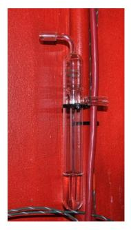
Figure 8-16: Image of water bubbler used for east beam port experiments.
