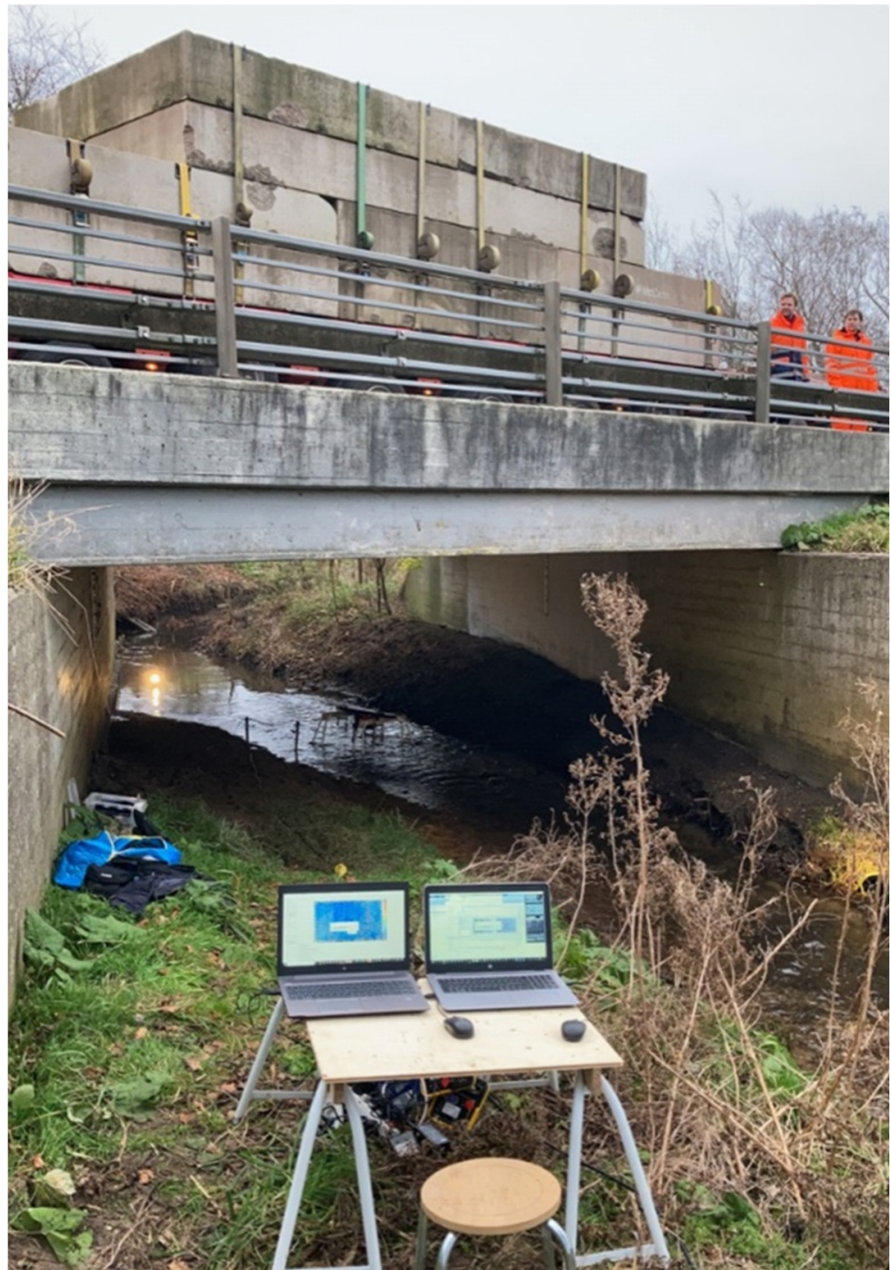
Figure 7. Real-time DIC setup for field testing.
