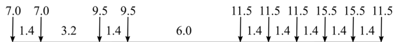
Figure 6. Axle load distribution for a class 100 vehicle in the Danish classification system [21], axle loads in tons and spacing in meters.
