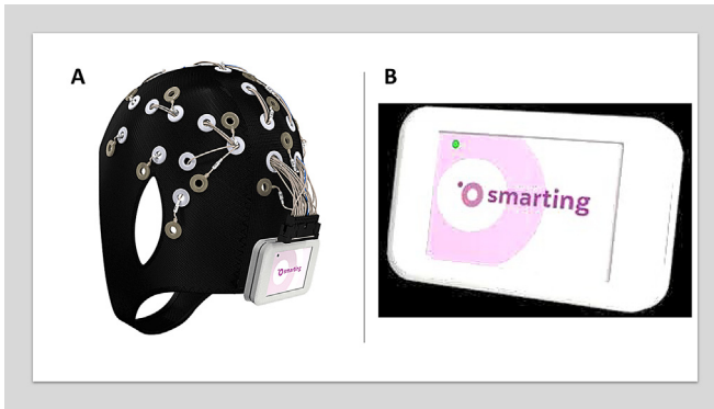
Fig. 3. Laboratory Resources of the Neuroengineering and Neuroacoustics Research Group. (A) MBrainTrain cap with 24 Ag/AgCl electrodes. (B) Smarting device used for communication between electrodes and recording device by means of Bluetooth.
