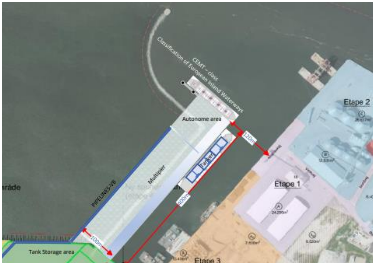
Figure 4 – Port of Vordingborg multiuse pier for autonomous bulk carriers
