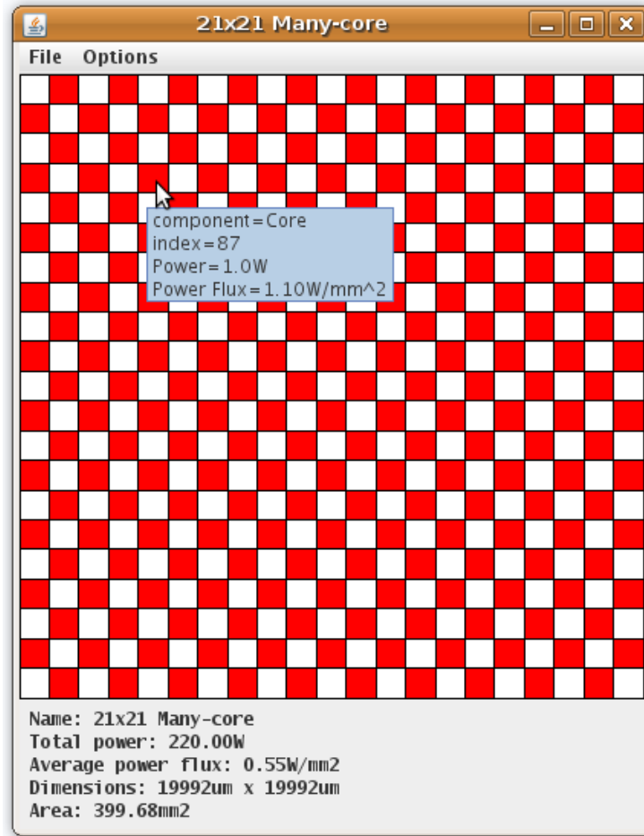
Figure 12: 21x21 many-core floorplan viewed in the floorplan viewer of HotSpotJ. Red boxes denote the cores and white boxes are the cache modules. The GUI displays information about a box as a tooltip when the mouse pointer is held steady over it.
