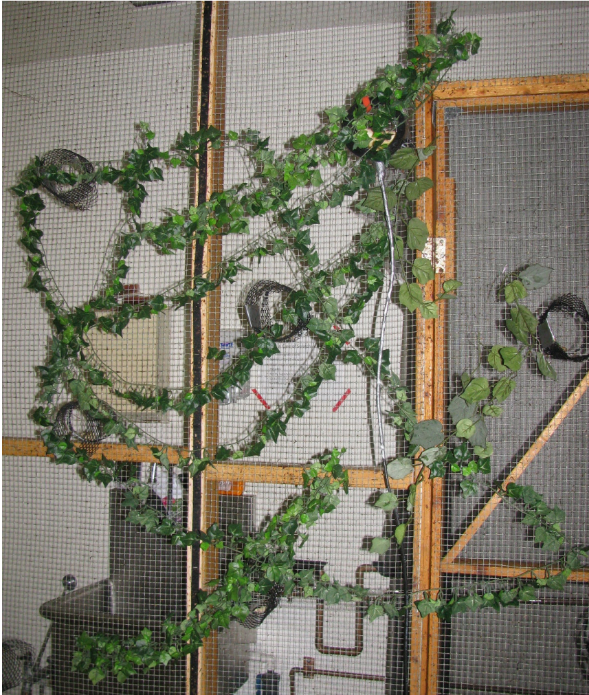
Figure 3.1. Experimental set-up to which bats were exposed-- feeders covered with artificial vegetation. The circular PIT-tag reader antenna is visible near the top of the photo.
