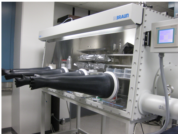
Figure 2.7: Argon-filled glove box for Li-ion battery assembly.
