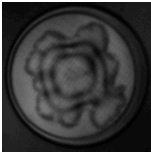
Figure 4.15: Fabry-Perot fringe photograph of third battery made using a 150 \mu m diameter membrane MEMS chip.
