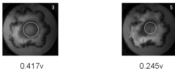
Figure 5.6: Fabry-Perot fringe images from the discharge cycle of the first experiment.
