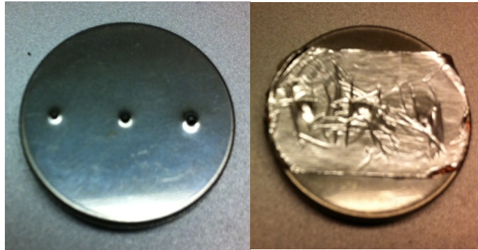
Figure 2.14: Pierced coin cell can (left). Assembled and taped cell (right).
