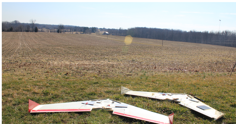
Figure 7.1: Two Procerus UAVs with 60 inch wingspans.
