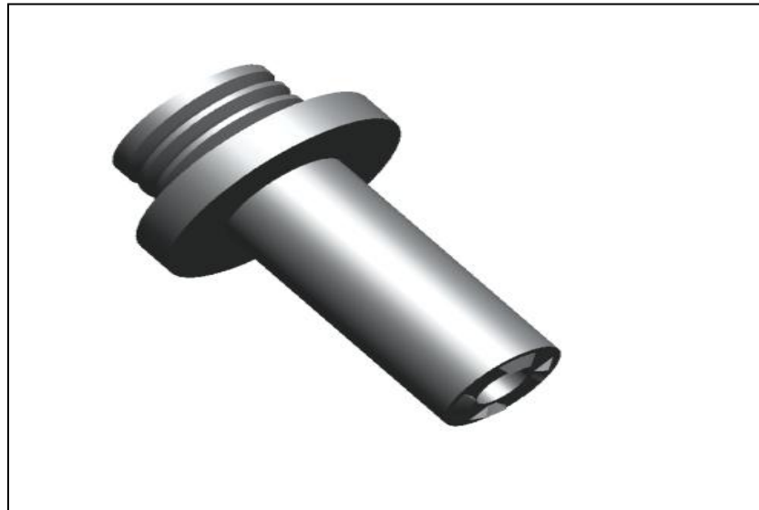
Figure 74. CAD Representation of Staking Tool
