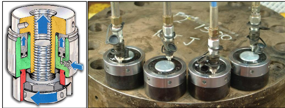
Figure 46. Left: Sketch of Cross Section of SKF Hydraulic Nut, Right: SKF Hydraulic Nut in Application
