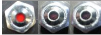
Figure 13. Color Match of Visual indicating fasteners (Red: No Load, Dark Red: 50% Load; Black: 100% Design Load)
