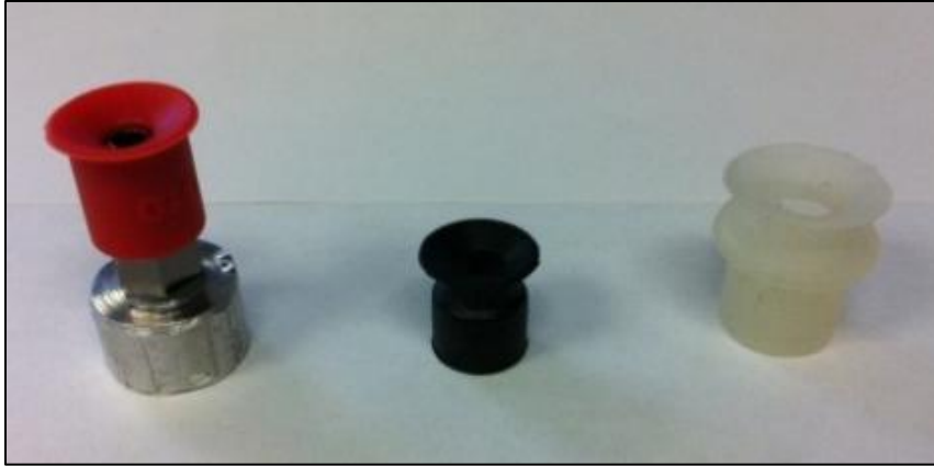
Figure 64. Left: Silicone Suction Cup, Middle: Nitrile Suction Cup, Right: Translucent Silicone Suction Cup After choosing the correct suction cup and the SMC actuator, the hand sketch for this subsystem was drawn and put in ProEngineer. After doing the embodiment design of this subsystem, the actual prototype is fabricated. This process is shown in the following pictures.
