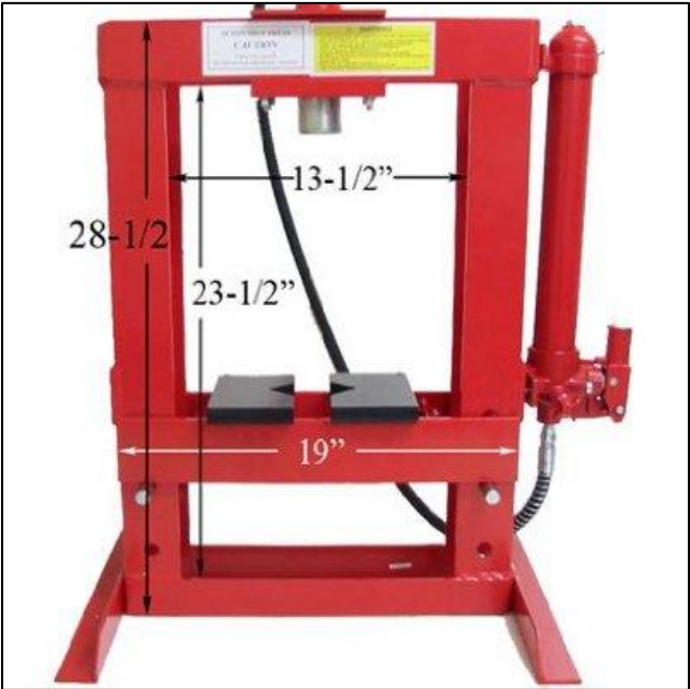
Figure 78. Overall Dimensions of H-Frame Bench Top Press
