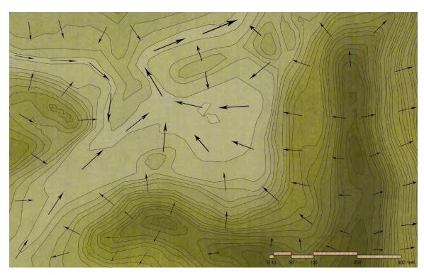
Fig 3.29 | Northeast corner detail, Contours with drainage arrows Image by author
