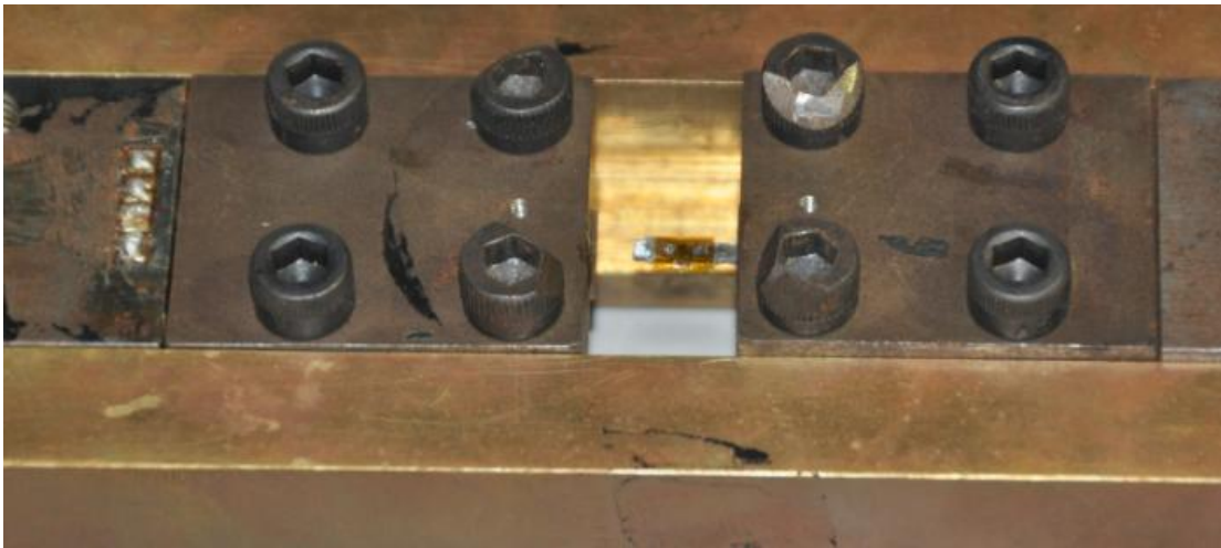
Figure 25: Fractured Sample of Dogbone Cut from Rolled Sheet of Polycrystalline \text{Fe}_{81}\text{Ga}_{19} + 1.0\% \text{NbC}
