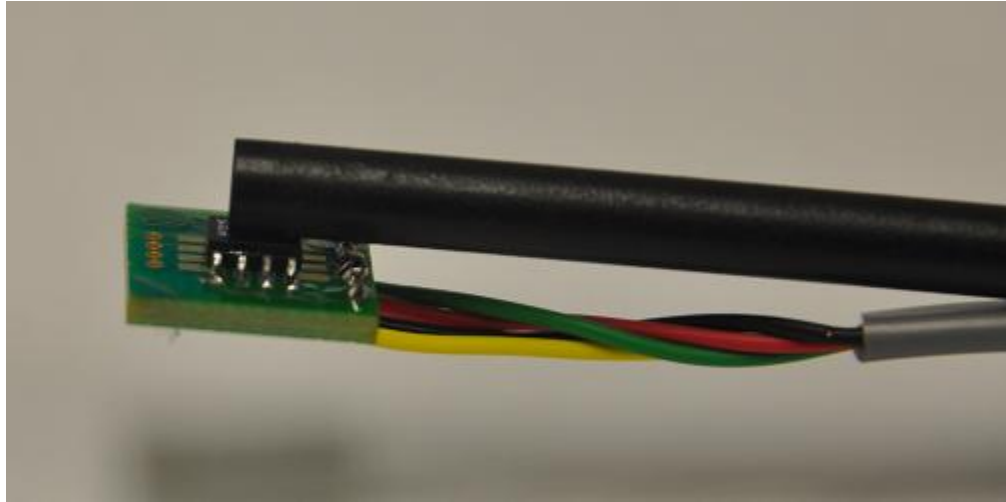
Figure 32: Calibrating NVE AAL002-02 GMR Sensor with Gaussmeter Probe
