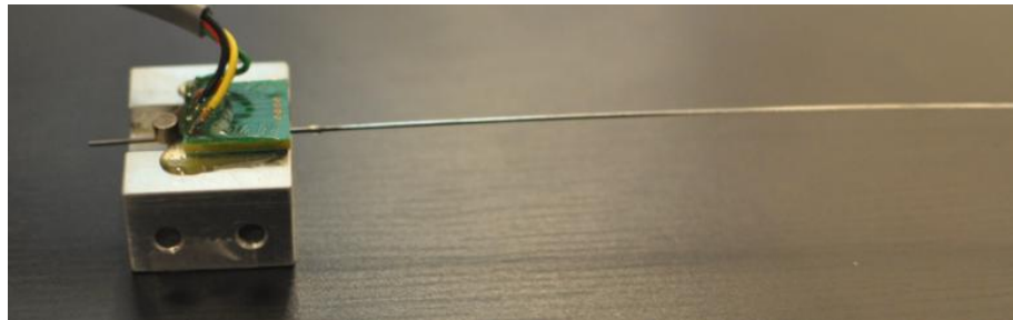
Figure 39: Prototype Whisker Sensor with Close Placement of Bias Magnet
