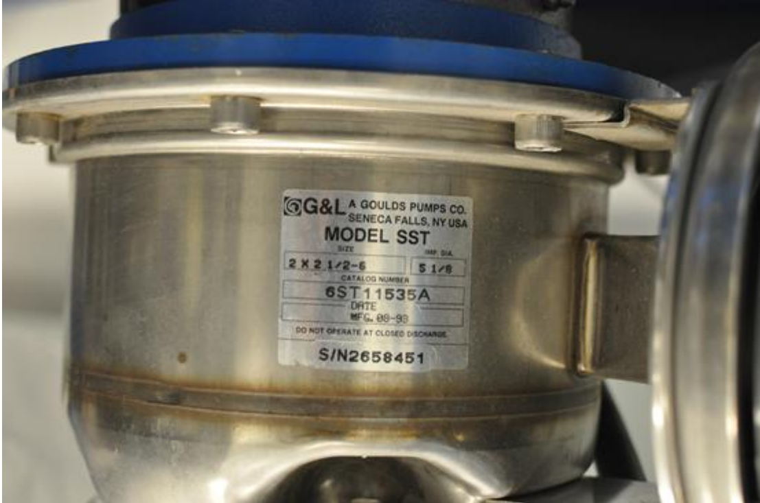
Figure 78: Water Tunnel Pump
