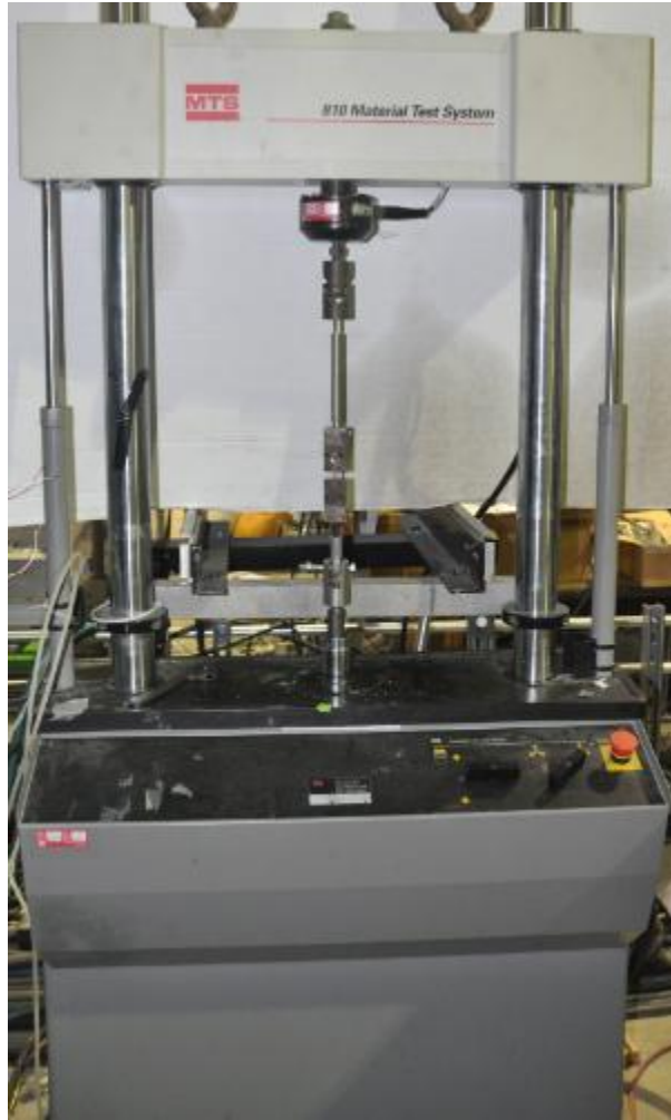
Figure 52: Material Test System for Tensile Tests of Galfenol Dogbone
