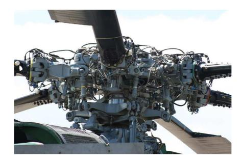
Figure 1.2: Example of swashplate with many parts (Source: www.fightercontrol.co.uk).
