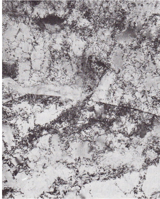
Figure 5. Heavily deformed aluminum microstructure [9]
