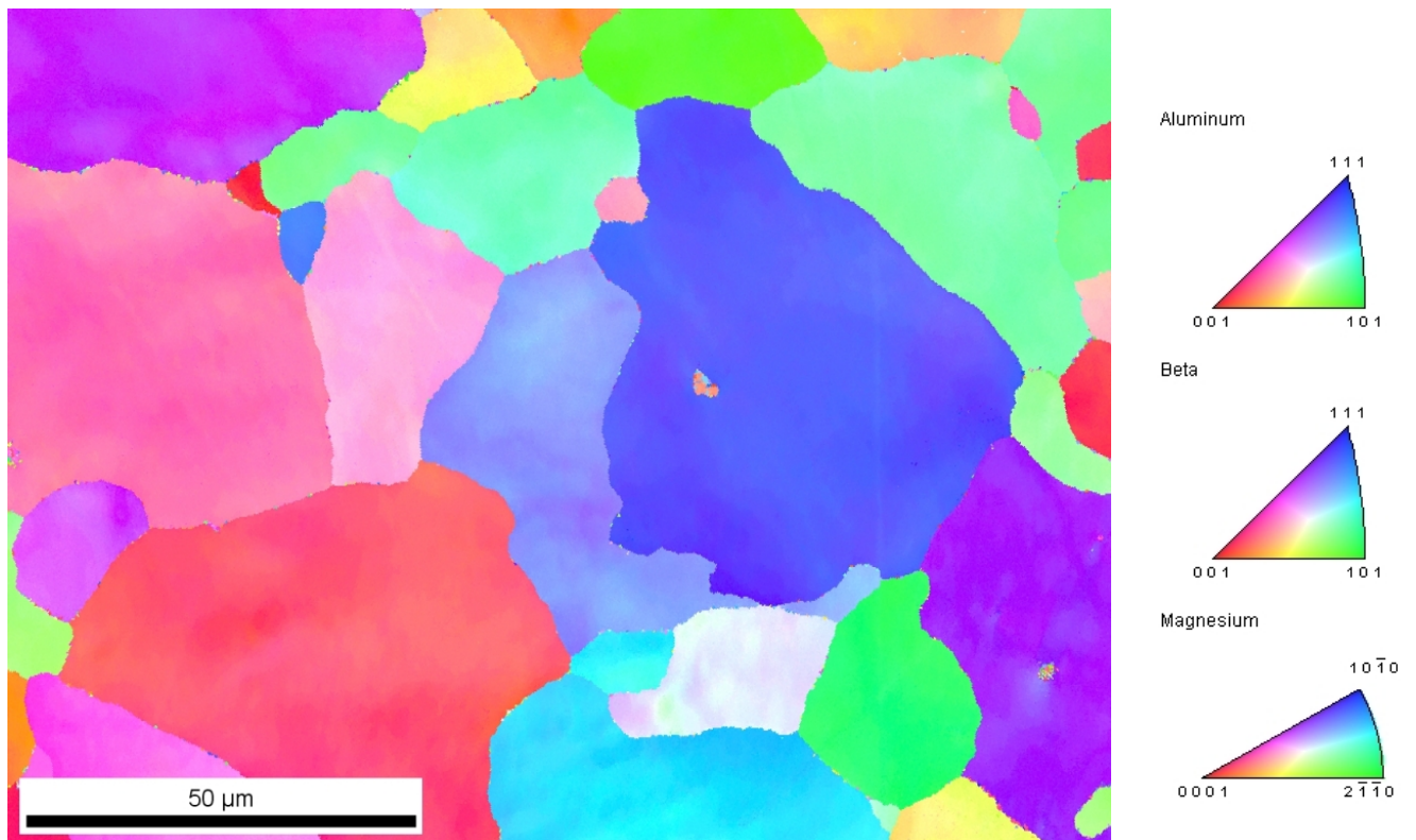
Figure 21. Inverse pole figure of untreated sensitized 5456 aluminum at 500X in the planar orientation
