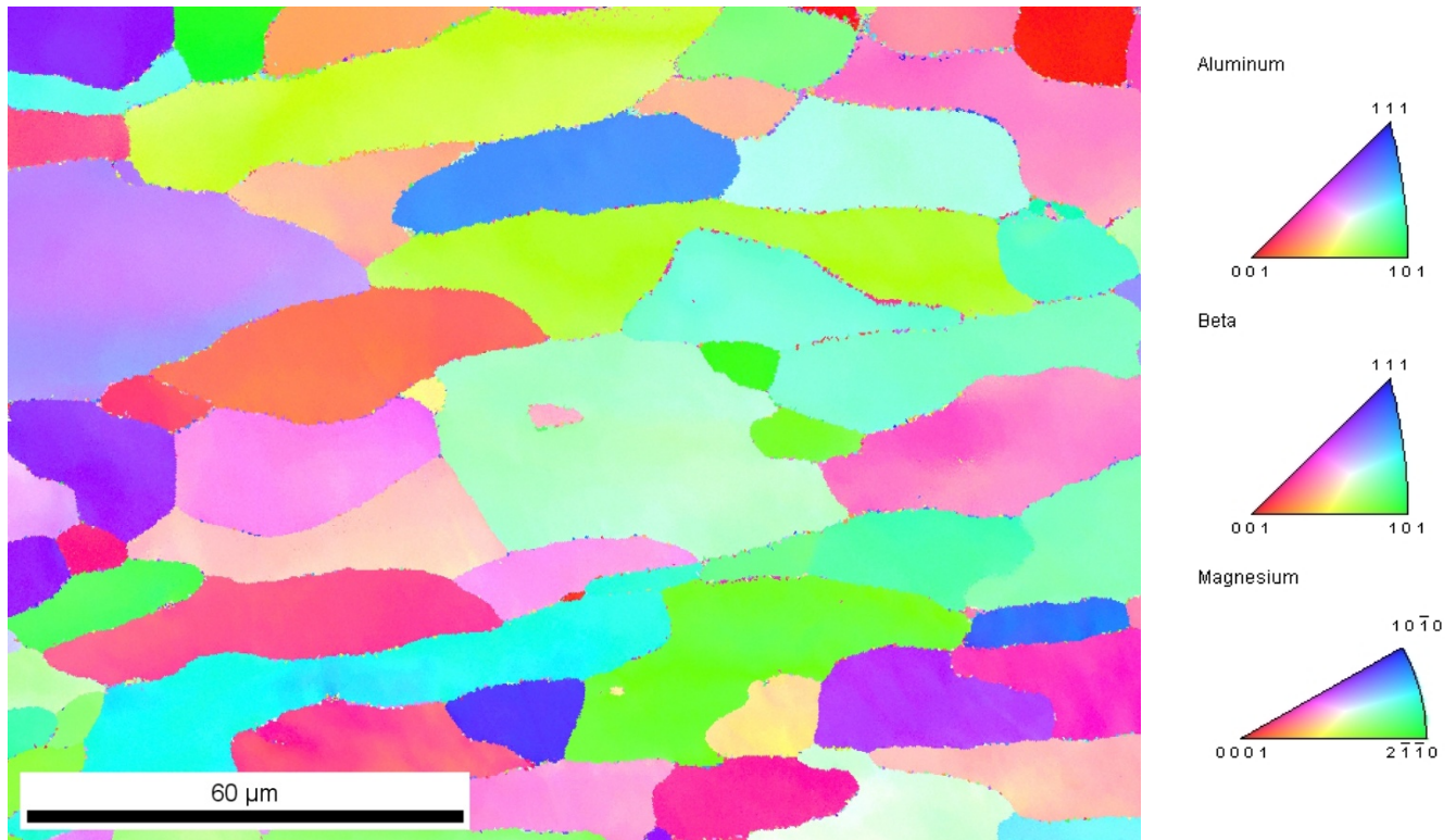
Figure 28. Inverse pole figure of UIT treated sensitized 5456 in the transverse orientation at 500X
