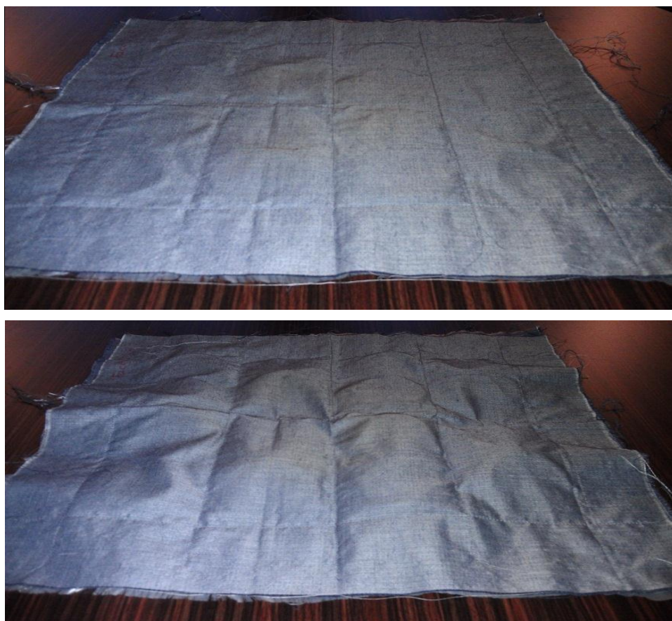
Figure 2.9: Typical expanding layer for inactivated (top) and activated (bottom) conditions
