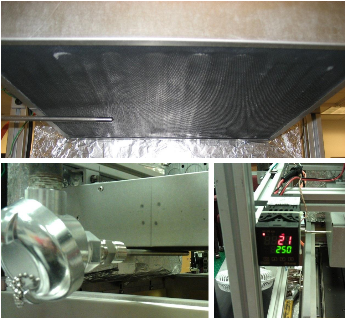
Figure 2.5: Radiant panel (top), thermocouple probe (bottom-left), and temperature controller (bottom-right) used to produce variable thermal exposures
