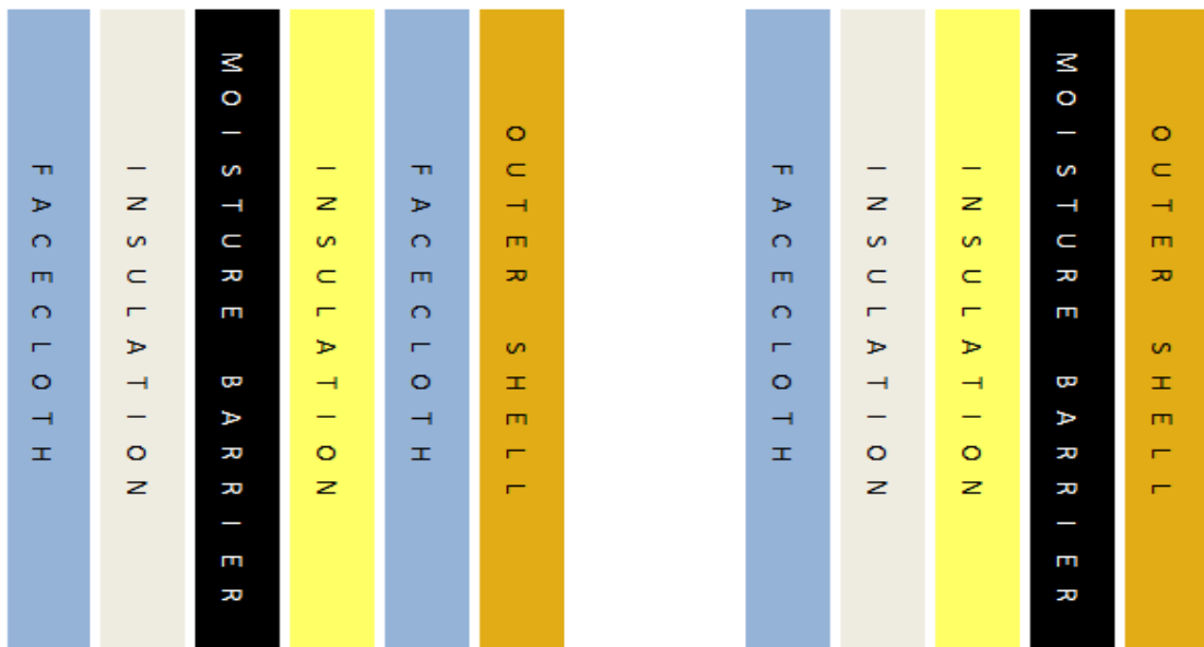
Figure 1.1: Layers constituting a split (left) and traditionally (right) layered garment of firefighter protective clothing
