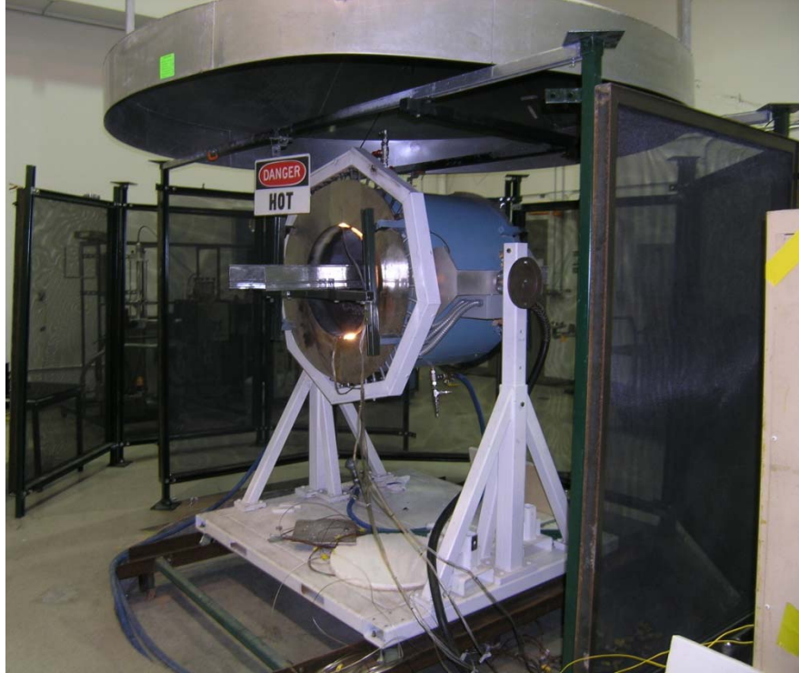
Figure 15. Photograph of Penlight small-scale radiant heat apparatus shown during startup testing for the DESIREE-Fire project, without cables in apparatus [Nowlen and Wyant 2008]
