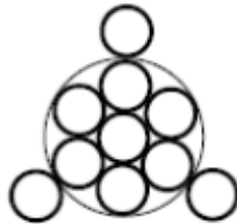
Figure 13. EPRI/NEI cable bundle [LaChance, Nowlen, Wyant, and Dandini 2003]
