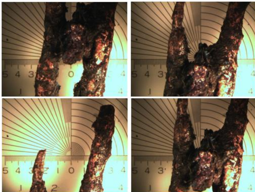
Figure 135: Radiation, Romex 12-2, Non Energized (Test No. 1)
