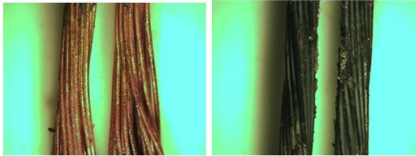
Figure 75: Direct Flame, Multi-strand 16-2, Non Energized (Test No. 19)
