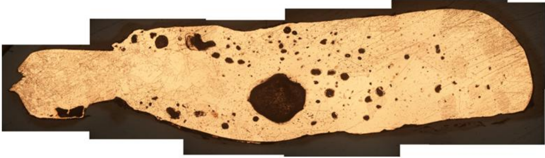
Figure 9: Compartment Tests, ROMEX 12-2, Non Energized (Sample # 40)
