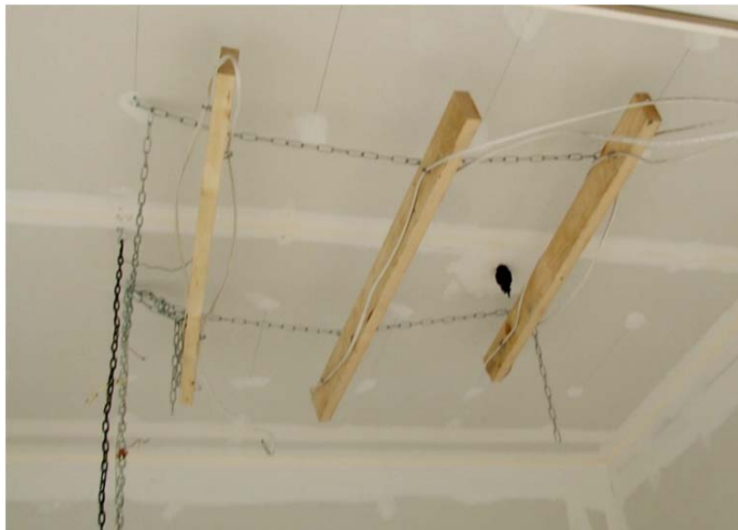
Figure 3-6: Wire Samples in the Ceiling with Thermocouple Tree-Full-Scale Compartment Tests (FSC)
