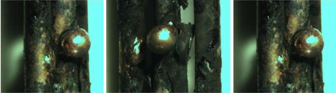
Figure 55: Direct Flame, ROMEX 12-2, Loaded (Test No. 14)
