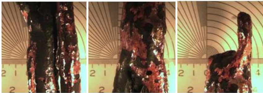
Figure 38: Compartment Tests, ROMEX 14-2, Loaded (Test No. 18)
