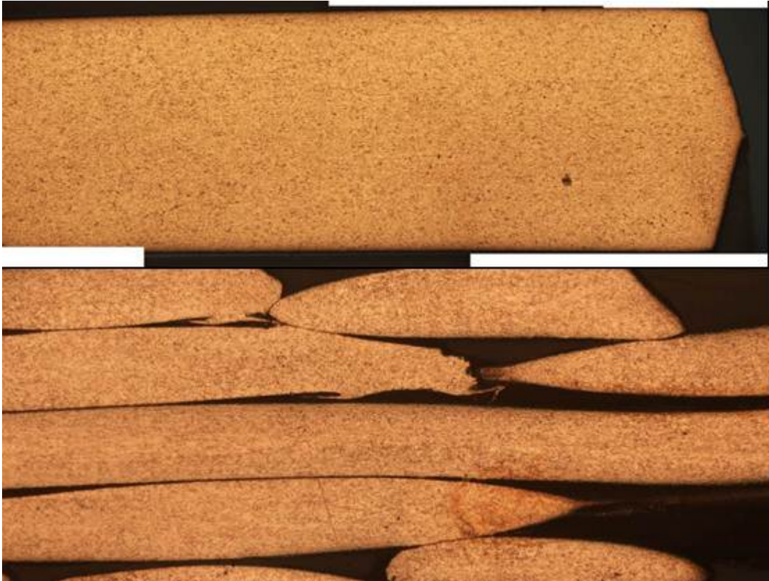
Figure 4-30: Grain Structures of Wire Control Samples (Unexposed Wires: Solid (Top) and Stranded (Bottom))
