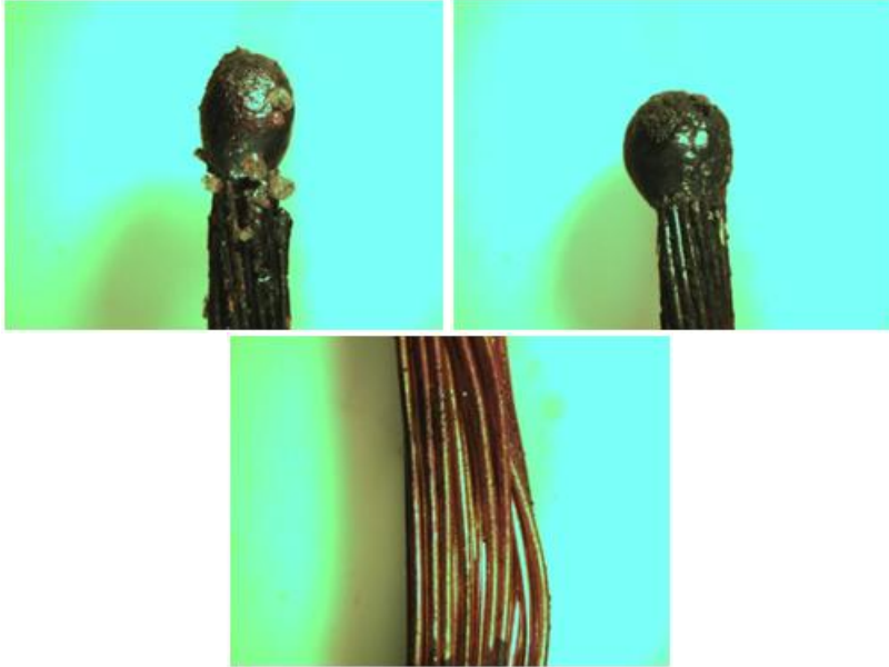
Figure 79: Direct Flame, Multi-strand 16-2, Non Energized (Test No. 23)
