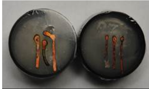
Figure 4-20: Mounted Samples (Cut and Etched)
