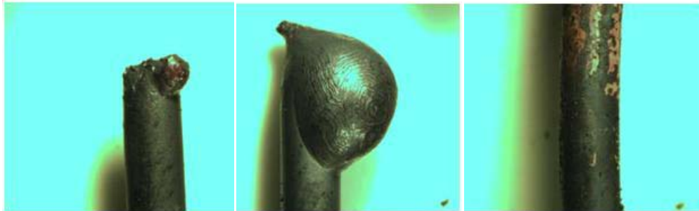
Figure 43: Direct Flame, ROMEX 12-2, Non Energized (Test No. 2)
