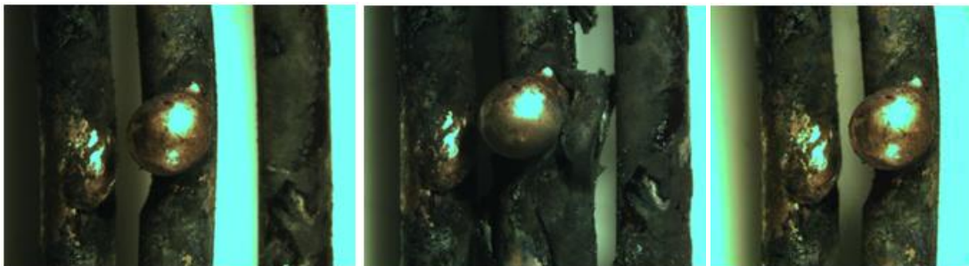
Figure 54: Direct Flame, ROMEX 12-2, Loaded (Test No. 13)
