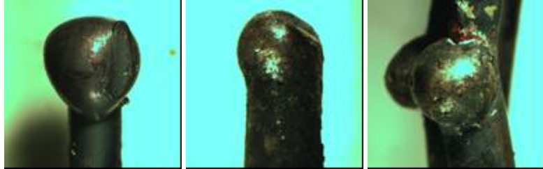
Figure 4-16: Beads Produced with Direct Flame Exposure (12-gauge: NE, E (center), and L)
