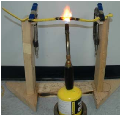
Figure 3-2: Direct Flame Testing Setup (DF)
