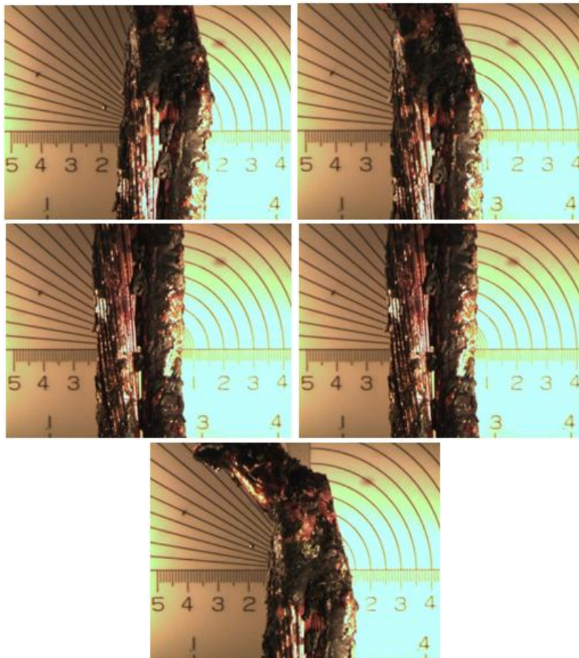
Figure 121: Radiation, Multi-strand 16-2, Non Energized (Test No. 2)
