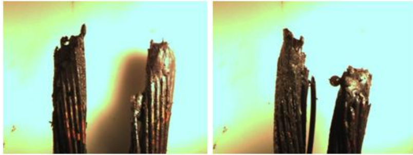
Figure 92: Direct Flame, Multi-strand 18-2, Non Energized (Test No. 37)
