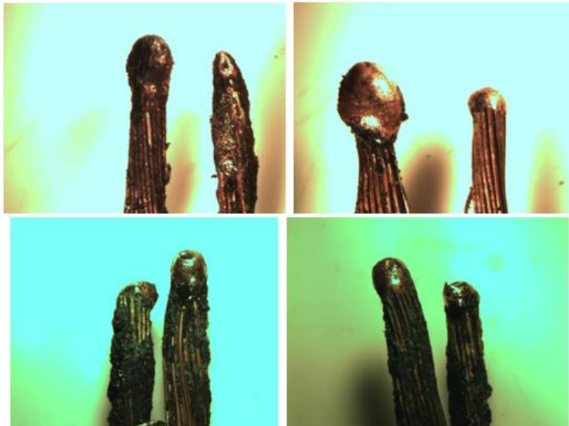
Figure 106: Direct Flame, Multi-strand 18-2, Loaded (Test No. 53)
