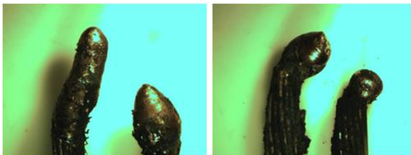
Figure 81: Direct Flame, Multi-strand 16-2, Energized (Test No. 25)
