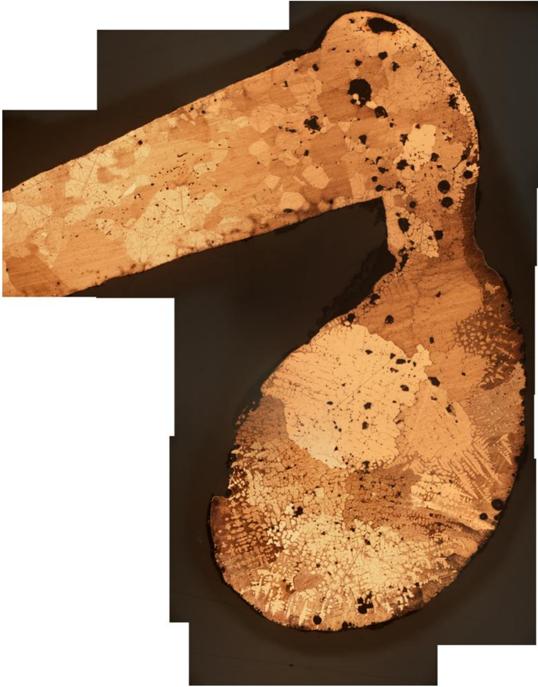
Figure 11: Compartment Tests, ROMEX 12-2, Loaded (Sample # 42)
