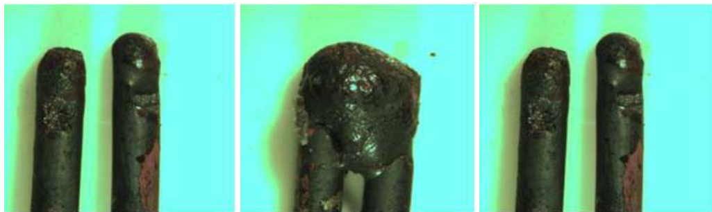
Figure 61: Direct Flame, ROMEX 14-2, Non Energized (Test No. 57)
