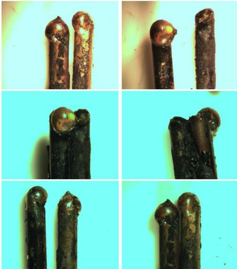
Figure 74: Direct Flame, ROMEX 14-2, Loaded (Test No. 72)
