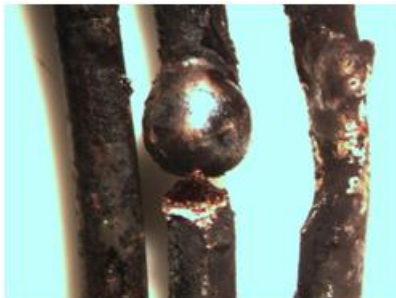
Figure 67: Direct Flame, ROMEX 14-2, Energized (Test No. 65)
