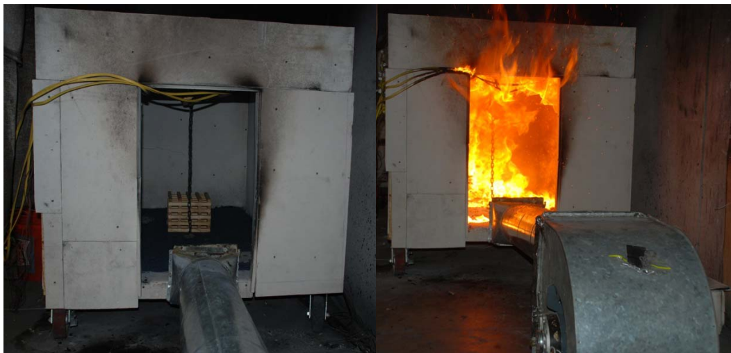
Figure 3-5: Flashover Scaled Compartment (SC)
