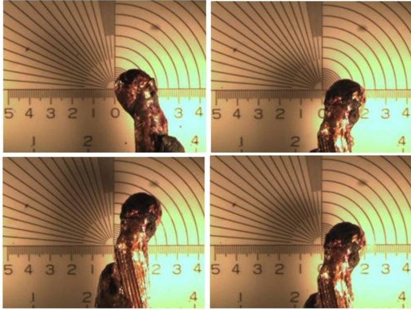
Figure 120: Radiation, Multi-strand 16-2, Non Energized (Test No. 1)
