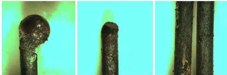
Figure 61: Direct Flame, ROMEX 14-2, Non Energized (Test No. 57)
