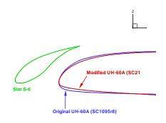
Figure 4.9: Modified UH60 Blade with Slat S-6
