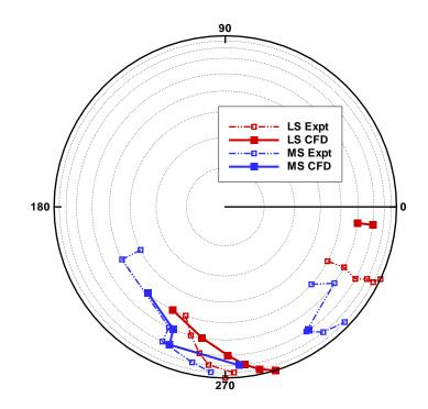
Figure 3.39: Lift stall (LS) and Moment stall (MS) map on the UH-60A rotor.
