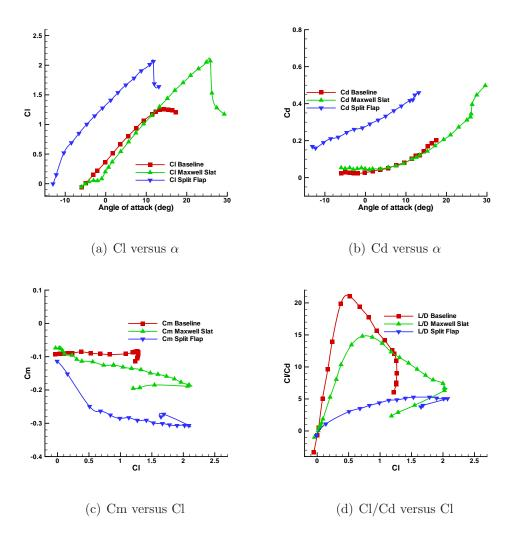
Figure 1.5: Airloads on Clark Y wing with split flap and Maxwell slat [7]
