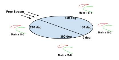
Figure 4.16: Schematic of slat actuation over a rotor revolution with appropriate phase offset.
