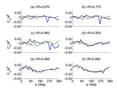
Figure 4.37: Time history of CFD pitching moments with dynamic slat actuations. Blue solid: no slat; Green dash: 1/rev dynamic slat; Red dash dot: up to 3/rev dynamic slat; Black dot: up to 5/rev dynamic slat
