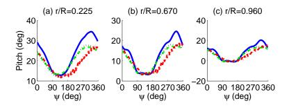
Figure 4.22: Variation of the effective geometric angle of attack as a function of azimuth at different radial stations. Blue solid: no slat; Green dash: steady slat S-6; Red dash dot: dynamic slat; Black dot: steady slat S-1.
