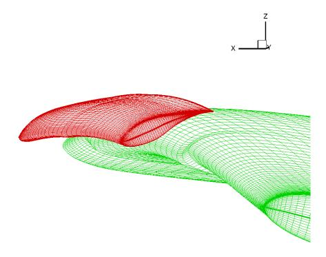
Figure 2.7: Slat deformation
