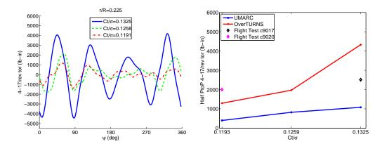
(a) CFD predicted Torsional 4-17/rev mo- (b) Half peak-to-peak 4-17/rev torsional ment vs azimuth ( $\Psi$ ) moments vs  $C_T/\sigma$
