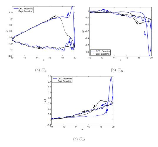
Figure 3.20: Periodic variation of the non-dimensional lift and pitching moment coefficients as a function of angle of attack for the baseline 2-D airfoil element,  $M_{\infty} = 0.3, k = 0.07, \alpha = 15^{\circ} - 5^{\circ} \cos(\omega t).$
