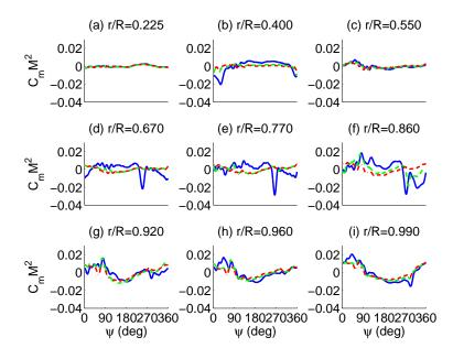
Figure 4.3: Variation of CFD pitching moments with thrust. Blue solid:  $C_T/\sigma = 0.1325$ ; Green dash:  $C_T/\sigma = 0.1258$ ; Red dash-dot:  $C_T/\sigma = 0.1190$
