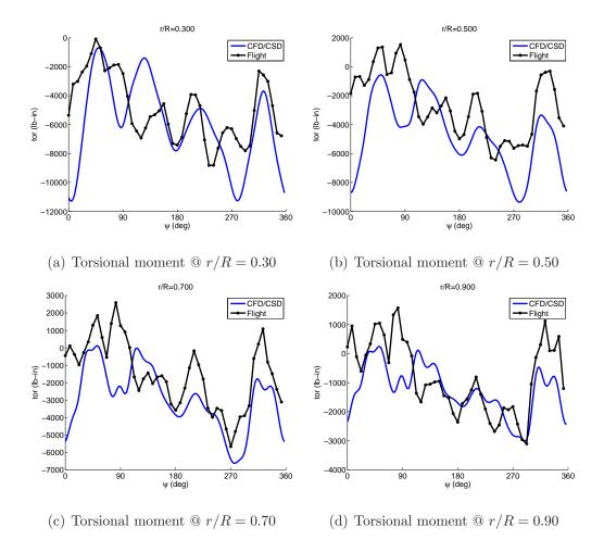
Figure 3.48: Comparison of CFD/CSD predicted sectional torsional moments with C9017 flight test data.
