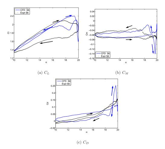
Figure 3.23: Periodic variation of the non-dimensional lift, pitching moment and drag coefficients as a function of angle of attack for the multi-element airfoil with the slat at S-6 configuration,  $M_{\infty} = 0.3$ , k = 0.07,  $\alpha = 15^{\circ} - 5^{\circ} \cos(\omega t)$  [53].
