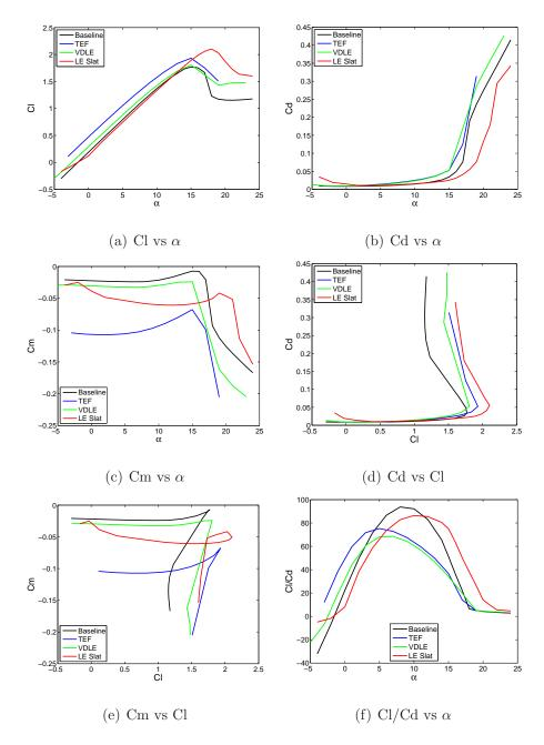
Figure A.2: Comparing airloads on various high lift devices ( $M = 0.3, Re = 4.14 \times 10^6$ )
