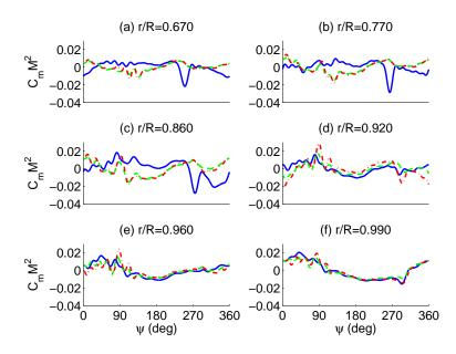
Figure 4.41: Variation of predicted pitching moment with thrust setting; Blue solid:  $C_T/\sigma = 0.1325$  baseline; Green dash:  $C_T/\sigma = 0.1391$  with S-6; Red dash dot:  $C_T/\sigma = 0.1458$  with S-6
