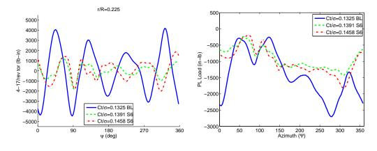
(a) CFD predicted (4 - 17/rev) torsional (b) CFD predicted Pitch link load vs azload vs azimuth ( $\Psi$ ) imuth ( $\Psi$ )
