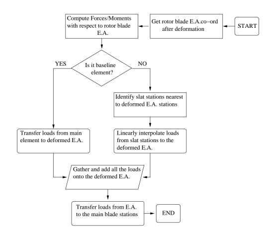
Figure 2.9: Flow Chart describing force transfer for Multi-element Rotor
