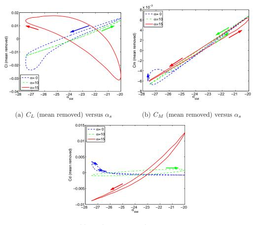
(c)  $C_D$  (mean removed) versus  $\alpha_s$
