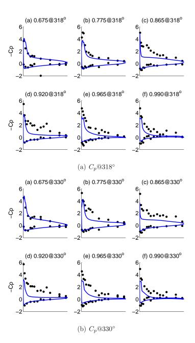
Figure 3.46: Surface pressure coefficient at different radial stations near *second* lift stall event for the baseline UH-60A rotor in C9017 flight condition. Black dot: Flight test data, Blue solid: CFD-CSD with shaft-fixed trim.
