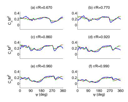
Figure 4.17: Time history of CFD normal loads with dynamic slat. Blue solid: no slat; Green dash: steady slat S-6; Red dash dot: steady slat S-1; Black dot: dynamic slat.
