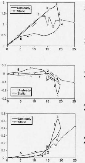
Stage 1: Airfoil exceeds static stall angle, flow reversals take place in boundary layer.
