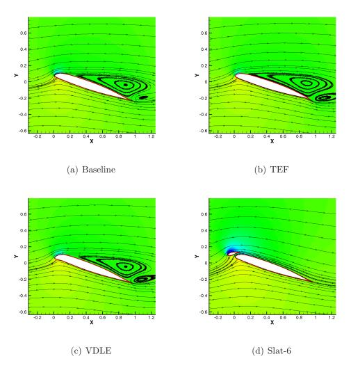
Figure A.6: Stream lines on various high lift devices at  $M=0.3, Re=4.14\times 10^6,$   $\alpha_{eff}=18.0^\circ$
