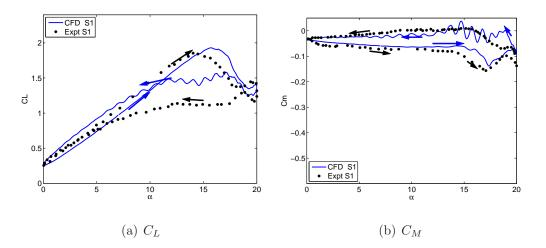
Figure 3.28: Periodic variation of the non-dimensional lift and pitching moment coefficients as a function of angle of attack for the multi-element airfoil with the slat at S-1 configuration,  $M_{\infty} = 0.4$ , k = 0.07,  $\alpha = 10^{\circ} - 10^{\circ} \cos(\omega t)$ .
