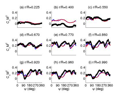
Figure 3.35: Time histories of the non-dimensional sectional normal forces at different radial stations along the span for the baseline UH-60A rotor in C9017 flight condition. Black dot: Flight test data, Blue solid: CFD-CSD with shaft-fixed trim, Red dash: CFD-CSD with free-flight trim.
