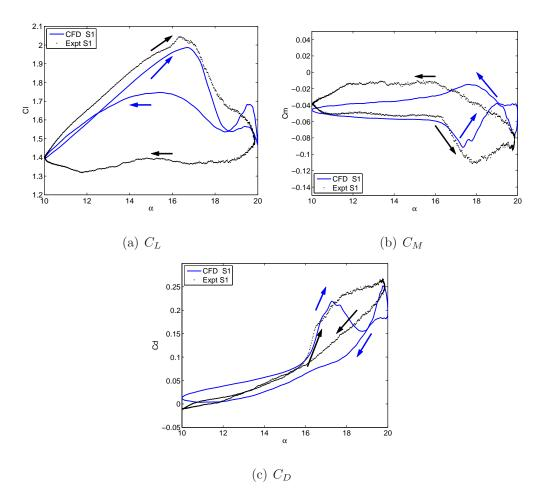
Figure 3.24: Periodic variation of the non-dimensional lift and pitching moment coefficients as a function of angle of attack for the multi-element airfoil with the slat at S-1 configuration,  $M_{\infty} = 0.3$ , k = 0.07,  $\alpha = 15^{\circ} - 5^{\circ} \cos(\omega t)$  [53].
