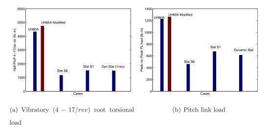
Figure 4.28: CFD/CSD predicted peak-to-peak vibratory root torsional and pitch link loads for various blade configurations.
