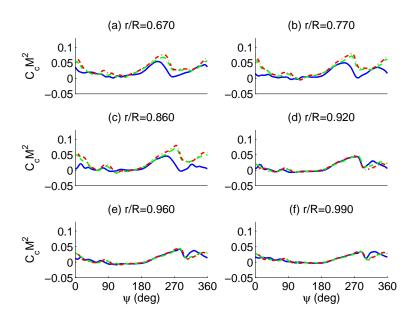
Figure 4.42: Variation of predicted chordwise force with thrust setting; Blue solid:  $C_T/\sigma = 0.1325$  baseline; Green dash:  $C_T/\sigma = 0.1391$  with S-6; Red dash dot:  $C_T/\sigma = 0.1458$  with S-6
