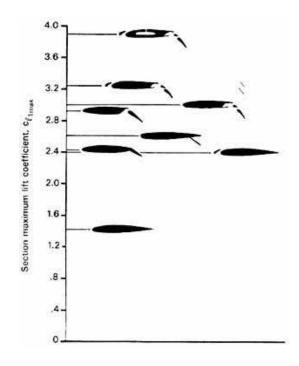
Figure 1.3: High-lift concepts. Courtesy NASA
