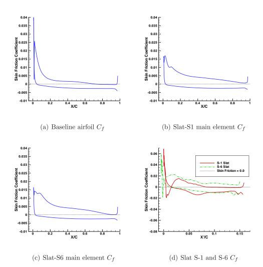
Figure 3.10: Skin friction coefficient  $(C_f)$  over the airfoil surface with and without the slat,  $Re = 4.14 \times 10^6$ ,  $M_{\infty} = 0.3$ ,  $\alpha = 15^{\circ}$ .
