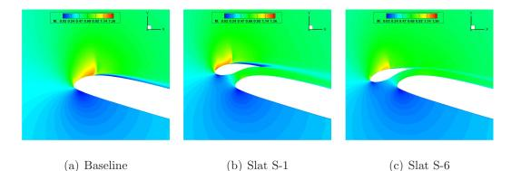
Figure 3.30: Mach contours on baseline and slatted airfoils at upstroke  $\alpha = 14.1^{\circ}$ during pitching cycle;  $M_{\infty} = 0.4$ , k = 0.07,  $\alpha = 10^{\circ} - 10^{\circ} \cos(\omega t)$ .
