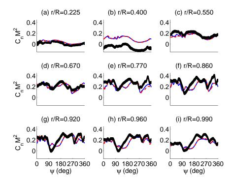
Figure 4.10: Predicted and measured sectional normal loads for C9017. Black dot: Flight Test Data; Blue solid: CFD UH60A Blade; Red dash: CFD UH60Amod Blade.
