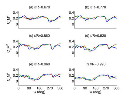
Figure 4.36: Time history of CFD normal loads all dynamic slat actuations. Blue solid: no slat; Green dash: 1/rev dynamic slat; Red dash dot: up to 3/rev dynamic slat; Black dot: up to 5/rev dynamic slat.
