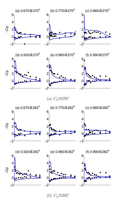
Figure 3.45: Surface pressure coefficient at different radial stations near *first* lift stall event for the baseline UH-60A rotor in C9017 flight condition. Black dot: Flight test data, Blue solid: CFD-CSD with shaft-fixed trim.
