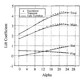
Figure 1.6: Lift contribution of flap and slat to total lift of an MEA airfoil. [5]
