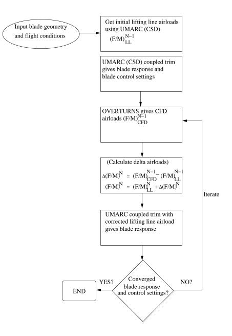
Figure 2.5: Loose Coupling Flow Chart
