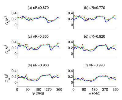
Figure 4.40: Variation of predicted normal loads with thrust setting; Blue solid:  $Ct/\sigma = 0.1325$  baseline; Green dash:  $Ct/\sigma = 0.1391$  with S-6; Red dash dot:  $Ct/\sigma = 0.1458$  with S-6
