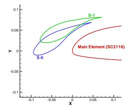
Figure 3.1: S-1 and S-6 slat configurations with respect to the baseline airfoil [55]. improvements.
