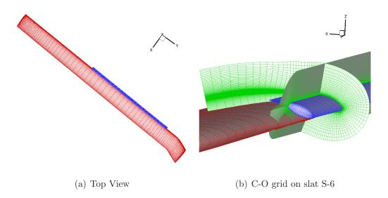
Figure 4.14: Slat S-6 Geometry
