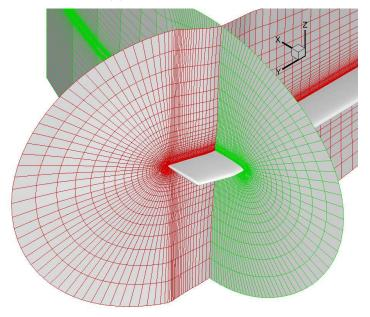
(b) C-O mesh at rotor tip
