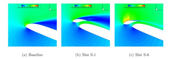
Figure 3.31: Mach contours on baseline and slatted airfoils at upstroke  $\alpha = 20^{\circ}$ during pitching cycle;  $M_{\infty} = 0.4$ , k = 0.07,  $\alpha = 10^{\circ} - 10^{\circ} \cos(\omega t)$ .
