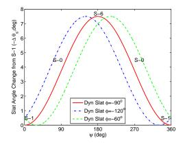
Figure 4.31: Time history of change of slat angle with respect to S-1 position over one cycle ( $\Delta \theta_s$  versus  $\psi$ ) due to three different phasing ( $\phi = -60^\circ, -90^\circ, -120^\circ$ ) of slat actuation
