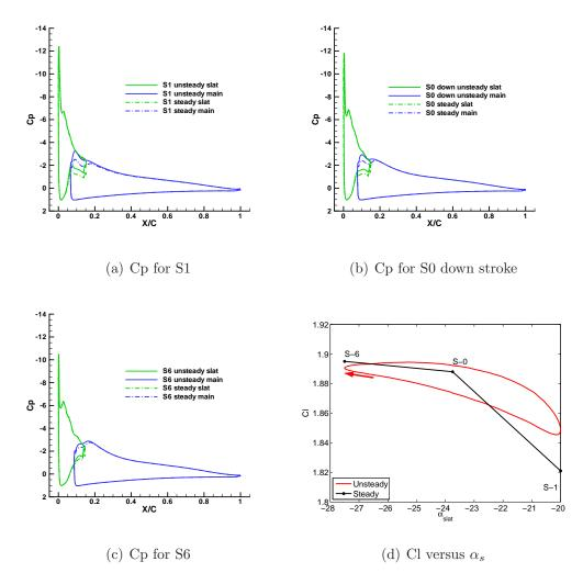
Figure B.4: Comparing Cp and lift values of unsteady slat on static main airfoil with steady values of the corresponding slat configurations at  $\alpha = 15^{\circ}$
