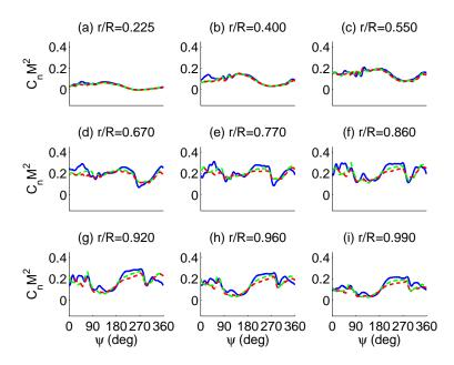
Figure 4.2: Variation of CFD normal loads with thrust. Blue solid:  $C_T/\sigma = 0.1325$ ; Green dash:  $C_T/\sigma = 0.1258$ ; Red dash-dot:  $C_T/\sigma = 0.1190$
