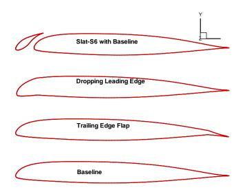
Figure A.1: Various high lift devices
