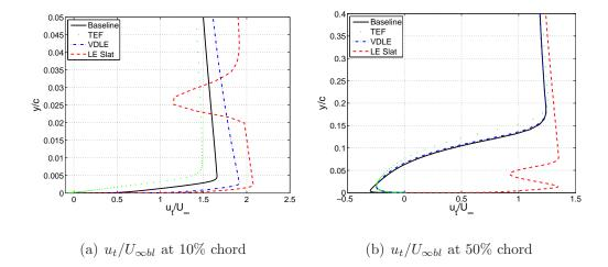
Figure A.5: Boundary layer profile on various high lift devices at M=0.3, Re= $4.14\times10^{6}, \, \alpha_{eff}=18.0^{\circ}$
