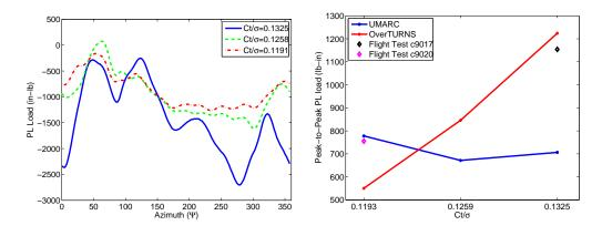
(a) CFD predicted Pitch link load vs az- (b) Half peak-to-peak pitch link load vs imuth ( $\Psi$ )  $C_T/\sigma$
