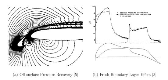
Figure 1.8: Viscous Effects of Gap
