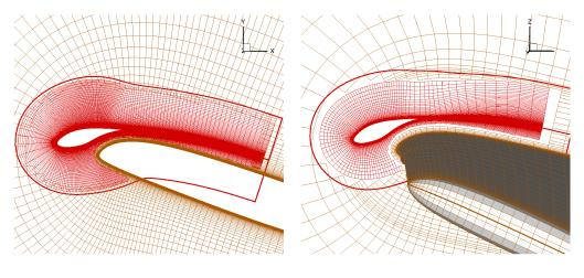
(a) 2-D hole-cutting for MEA (b) 3-D hole-cutting for MEA
