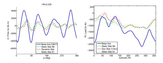
(a) CFD predicted (4 - 17/rev) torsional (b) CFD predicted Pitch link load vs azload vs azimuth ( $\Psi$ ) imuth ( $\Psi$ )
