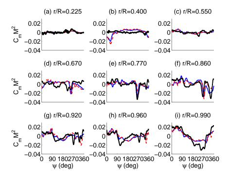
Figure 4.11: Predicted and measured sectional moment loads for C9017. Black dot: Flight Test Data; Blue solid: CFD UH60A Blade; Red dash: CFD UH60Amod Blade.
