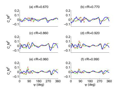
Figure 4.43: Variation of predicted normal (3-20/rev) loads with thrust setting; Blue solid:  $C_T/\sigma = 0.1325$  baseline; Green dash:  $C_T/\sigma = 0.1391$  with S-6; Red dash dot:  $C_T/\sigma = 0.1458$  with S-6
