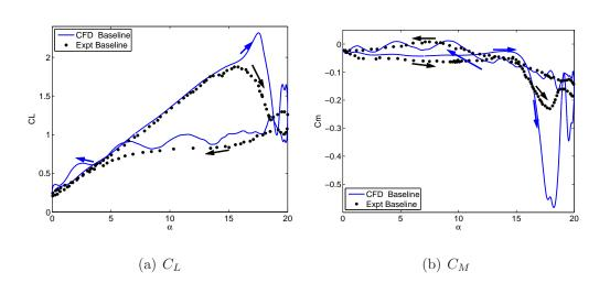
Figure 3.27: Periodic variation of the non-dimensional lift and pitching moment coefficients as a function of angle of attack for the baseline airfoil section,  $M_{\infty} =$ 0.4, k = 0.07,  $\alpha = 10^{\circ} - 10^{\circ} \cos(\omega t)$  [53].
