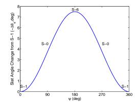
Figure 4.12: Time history of slat angle over one cycle  $(-\Delta \theta_s \text{ versus } \psi)$  due to 1/rev slat actuations
