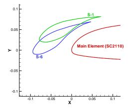
Figure 1.11: S-1 and S-6 slat configurations with respect to the baseline airfoil [55].
