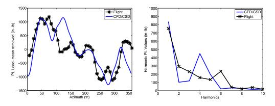
(a) Pitch link (mean removed) vs azimuth  $\psi$  (b) Pitch link harmonic amplitudes vs harmonics
