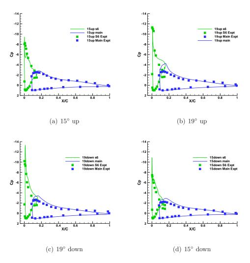
Figure 3.26: Surface pressure on Slat-S6 SC2110 airfoil at high angles [53].
