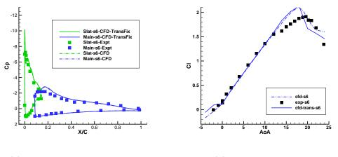
(a) Pressure Co-efficient at  $\alpha = 15^{\circ}$
