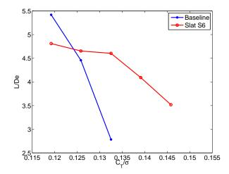
Figure 4.48: Comparing  $L/D_e$  for baseline rotor with that having slats S-6 and S-1
