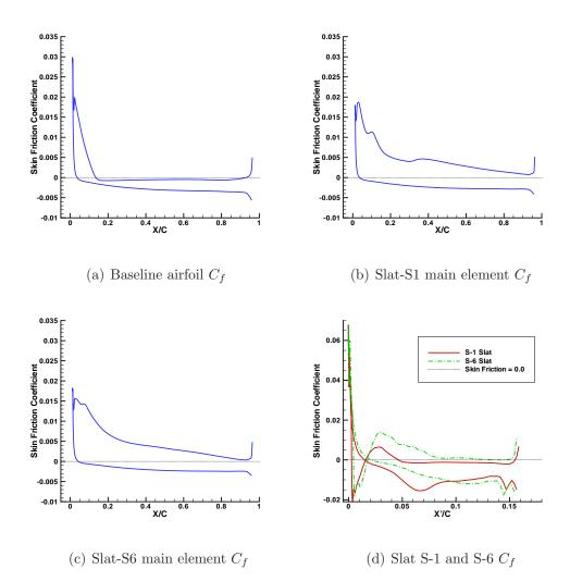
Figure 3.14: Skin friction coefficient  $(C_f)$  over the airfoil surface with and without the slat,  $Re = 4.14 \times 10^6$ ,  $M_{\infty} = 0.3$ ,  $\alpha = 18^{\circ}$
