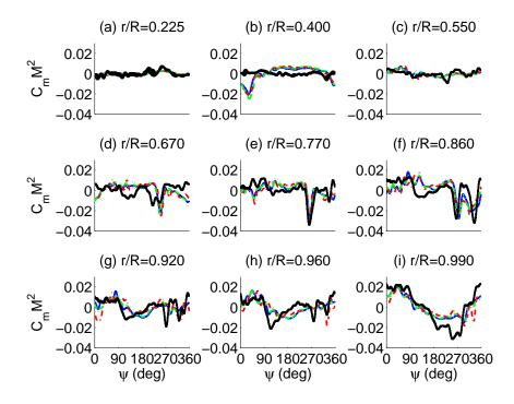
Figure 3.41: Time histories of the non-dimensional sectional pitching moment coefficients (means removed) at different radial stations along the span for the baseline UH-60A rotor in C9017 flight condition. Black dot: Flight test data, Blue solid: Grid size  $133 \times 130 \times 61$ , Green dash: Grid size  $133 \times 197 \times 61$ , Red dash-dot: Grid size  $133 \times 259 \times 61$ , Cyan dots: Grid size  $199 \times 130 \times 61$ .
