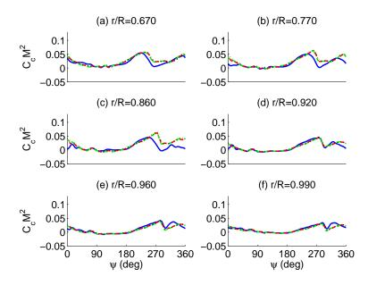
Figure 4.19: Time history of CFD chord wise forces with dynamic slat. Blue solid: no slat; Green dash: steady slat S-6; Red dash dot: steady slat S-1; Black dot: dynamic slat.
