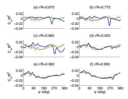
Figure 4.18: Time history of CFD pitching moments with dynamic slat. Blue solid: no slat; Green dash: steady slat S-6; Red dash dot: steady slat S-1; Black dot: dynamic slat.
