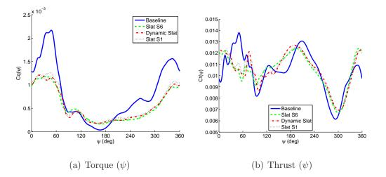
Figure 4.30: Non-dimensional torque and thrust time history over one rotor revolution.
