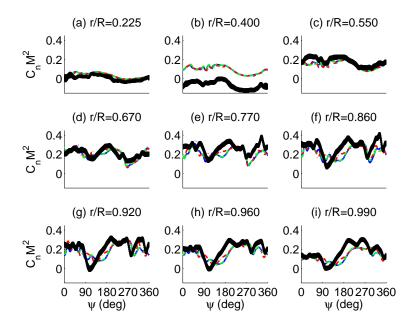
Figure 3.40: Time histories of the non-dimensional sectional normal forces at different radial stations along the span for the baseline UH-60A rotor in C9017 flight condition. Black dot: Flight test data, Blue solid: Grid size  $133 \times 130 \times 61$ , Green dash: Grid size  $133 \times 197 \times 61$ , Red dash-dot: Grid size  $133 \times 259 \times 61$ , Cyan dots: Grid size  $199 \times 130 \times 61$ .
