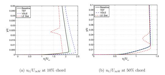
Figure A.4: Boundary layer profile on various high lift devices at  $M = 0.3, Re = 4.14 \times 10^6, \alpha_{eff} = 12.0^{\circ}$
