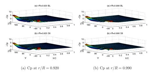
Figure 4.26: Mitigation of pressure peaks near leading edge of main blade due to slat S-6 outboard of slat.
