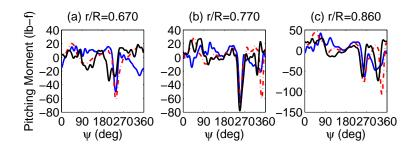
Figure 3.37: Time histories of sectional pitching moment coefficients (means removed) at three outboard radial stations for the baseline UH-60A rotor in C9017 flight condition taken from previous CFD-CSD work by Sitaraman et. al. [90]. Black solid : Flight test data, Blue solid: CFD-CSD with shaft-fixed trim, Red dash-dot: previous CFD-CSD with shaft-fixed trim.
