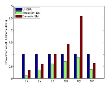
Figure 4.29: CFD predicted 4/*rev* Hub loads; no slat; Steady Slat S-6; Dynamic Slat
