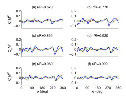
Figure 4.21: Time history of CFD vibratory normal loads (3 - 20/rev) with dynamic slat. Blue solid: no slat; Green dash: steady slat S-6; Red dash dot: steady slat S-1; Black dot: dynamic slat.
