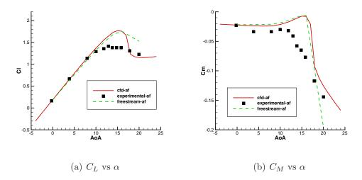
Figure 3.3: Effect of wind tunnel wall correction on lift and pitching moment coefficients of the main airfoil section,  $Re = 4.14 \times 10^6$ ,  $M_{\infty} = 0.3$ .
