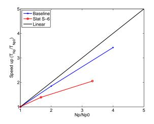
Figure 4.15: Computational time speed up for Np processors with respect to the corresponding minimum number of processors (Np0) used for baseline as well as slatted (S-6) rotors
