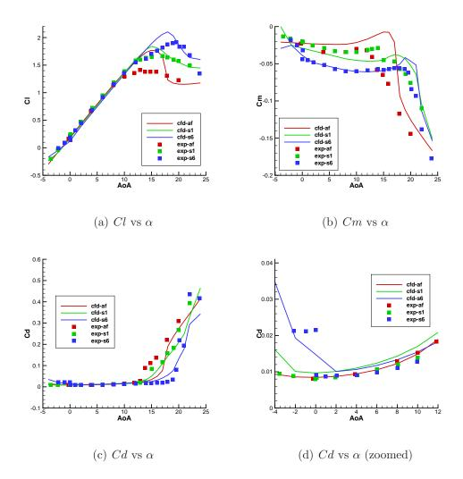
Figure 3.4: Steady airload validation on baseline airfoil and baseline with S-1 and S-6 slat configurations for  $Re = 4.14 \times 10^6$ ,  $M_{\infty} = 0.3$
