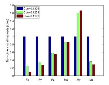
Figure 4.7: CFD predicted 4/rev Hub loads;  $C_T/\sigma$  = 0.1325;  $C_T/\sigma$  = 0.1258;  $C_T/\sigma$  = 0.119
