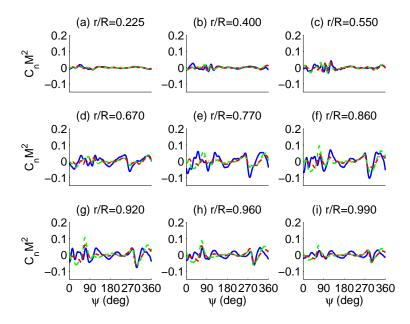
Figure 4.8: Variation of CFD vibratory normal loads (3 - 20/rev) with thrust. Blue solid:  $C_T/\sigma = 0.1325$ ; Green dash:  $C_T/\sigma = 0.1258$ ; Red dash-dot:  $C_T/\sigma = 0.119$
