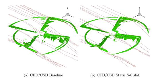
Figure 4.24: Comparison of Q-criterion iso-surface contours of baseline rotor with that having static S-6 slat.
