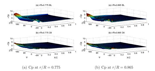
Figure 4.25: Mitigation of pressure peaks near leading edge of main blade due to slat S-6 in slat region.
