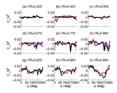
Figure 3.36: Time histories of the non-dimensional sectional pitching moment coefficients (means removed) at different radial stations along the span for the baseline UH-60A rotor in C9017 flight condition. Black dot: Flight test data, Blue solid: CFD-CSD with shaft-fixed trim, Red dash: CFD-CSD with free-flight trim.
