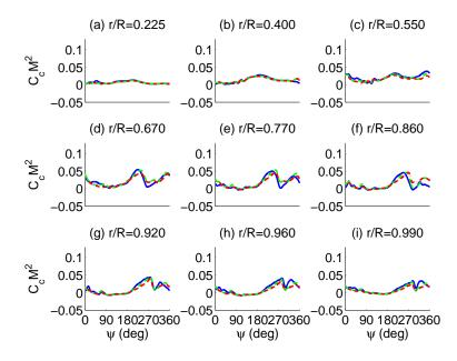
Figure 4.4: Variation of CFD chord wise forces with thrust. Blue solid:  $C_T/\sigma = 0.1325$ ; Green dash:  $C_T/\sigma = 0.1258$ ; Red dash-dot:  $C_T/\sigma = 0.1190$
