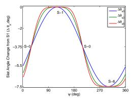
Figure 4.35: Slat actuation (up to 1, 3, 5/rev) with respect to S-1 position over one rotor revolution ( $\Delta \theta_s$  vs  $\psi$ )
