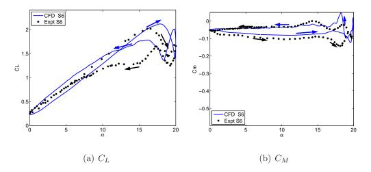
Figure 3.29: Periodic variation of the non-dimensional lift and pitching moment coefficients as a function of angle of attack for the multi-element airfoil with the slat at S-6 configuration,  $M_{\infty} = 0.4$ , k = 0.07,  $\alpha = 10^{\circ} - 10^{\circ} \cos(\omega t)$ .
