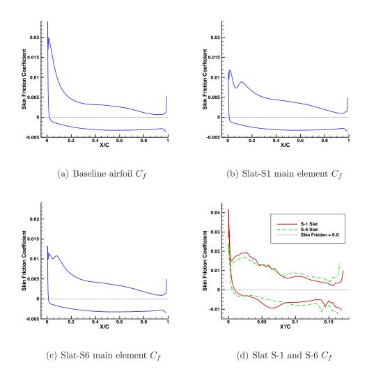
Figure 3.6: Skin friction coefficient  $(C_f)$  over the airfoil surface with and without the slat,  $Re = 4.14 \times 10^6$ ,  $M_{\infty} = 0.3$ ,  $\alpha = 10^{\circ}$ .
