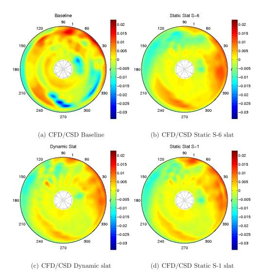
Figure 4.20: Comparison of the pitching moment variation across the rotor disk for the static and dynamic slat analyses with the baseline no-slat rotor.
