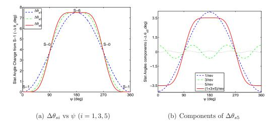
Figure 4.33: Time history of change of slat angle with respect to S-1 over one cycle ( $\Delta \theta_s$  versus  $\psi$ ) due to three (up to1, 3, 5/rev) slat actuations and build up of the  $\Delta \theta_{s5}$  slat actuation
