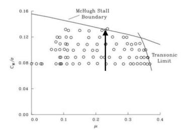
Figure 1.1: Thrust limit on a UH-60A rotor [1]
