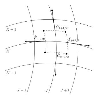
Figure 2.1: Schematic showing computational cell.
