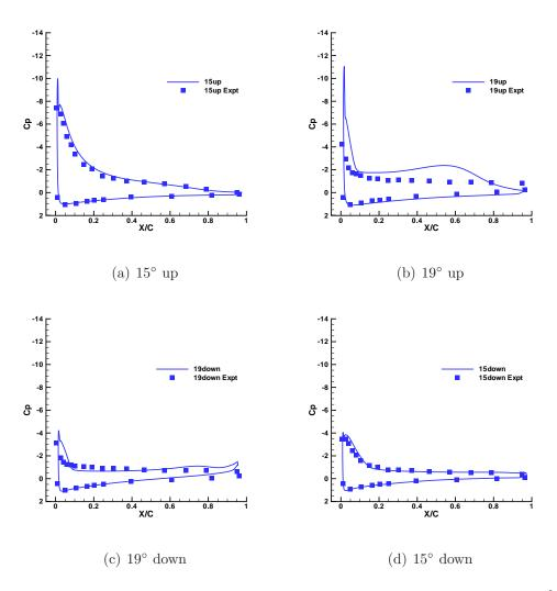
Figure 3.22: Surface pressure on baseline SC2110 airfoil near stall region [53].
