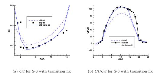
Figure 3.17: Effect of transition fix on slatted S-6 airfoil;  $Re = 4.14 \times 10^6, M_{\infty} = 0.3$
