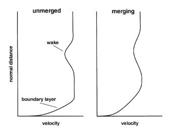
Figure 1.9: Process of formation of CBL in a typical multi-element airfoil [6].
