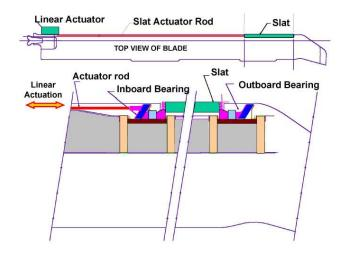
Figure 1.12: Elastomeric bearing concept for slat actuation [53].
