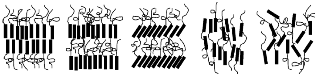
Figure 4.1. Illustration of molecular packing in possible rod-coil block copolymer microphases. From left to right the phases are bilayer, smectic A-like monolayer, smectic C-like monolayer, nematic, and isotropic. While regions of the lamellar, nematic, and isotropic phases can be clearly demarcated on the phase diagram, discerning between the lamellar structures is more difficult. On the basis of domain spacing, the two monolayer phases are the most probable lamellar morphologies, with transitions in rod tilt and chain stretching occurring as the polymers are heated through the order-disorder transition. 231 Reproduced from Segalman and coworkers.
