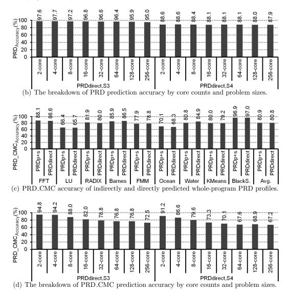
Figure 4.16: PRD profile prediction accuracy for scaling core count and problem size together.
