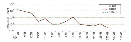
Figure 5.4: PRD profiles from the FFT benchmark running on 64 cores at the S2 problem size across 32K, 64K, and 128K per-core L2 capacity.
