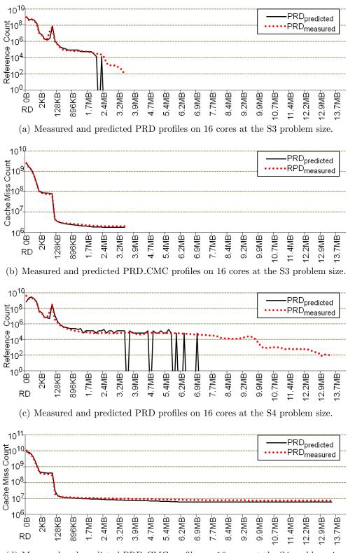
(d) Measured and predicted PRD\_CMC profiles on 16 cores at the S4 problem size.
