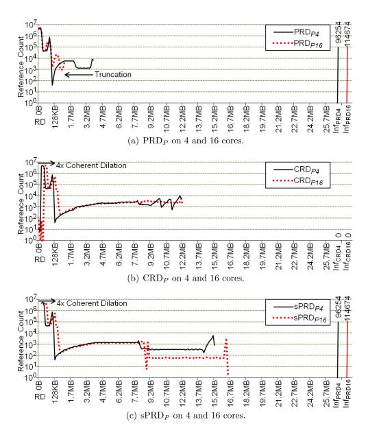
Figure 3.8: FFT's private-data locality profiles running on 4 cores and 16 cores at the S2 problem size.
