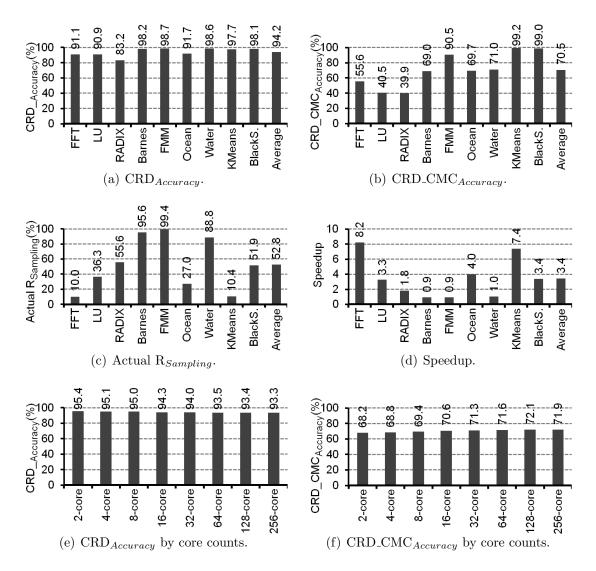
Figure 7.3: Accuracy and performance of the sampling technique with  $R_{Sampling} = 0.1$  and  $R_{Pruning} = 0.99$  for CRD profiles.
