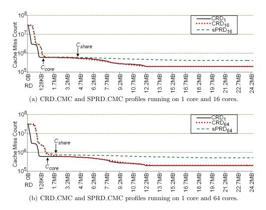
Figure 3.14: FFT's CMC profiles running on 1, 16, and 64 cores at the S2 problem size.
