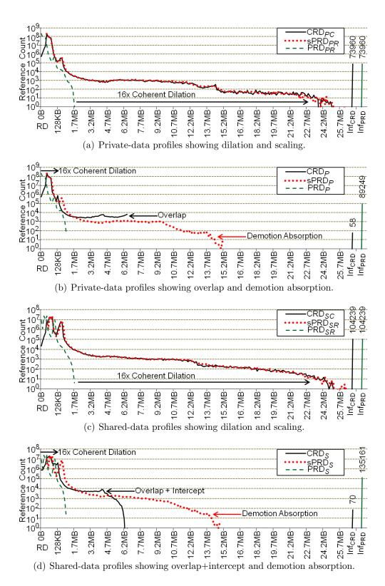
Figure 3.3: Barnes' locality profiles for the most important parallel region running on 16 cores at the S2 problem size.
