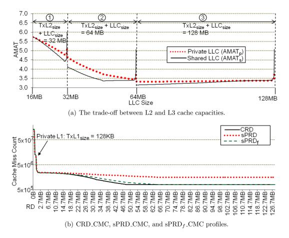
Figure 6.5: The trade-off between  $L2_{size}$  and  $LLC_{size}$  for FFT running on 16 cores at the S3 problem size.
