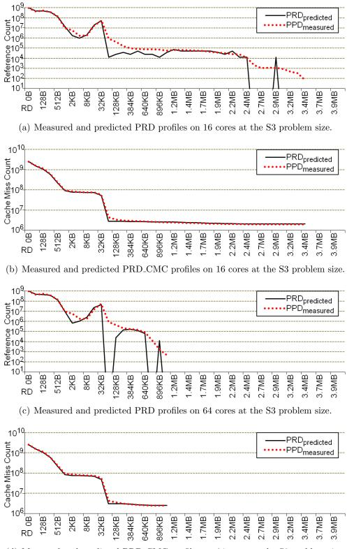
(d) Measured and predicted PRD\_CMC profiles on 64 cores at the S3 problem size.
