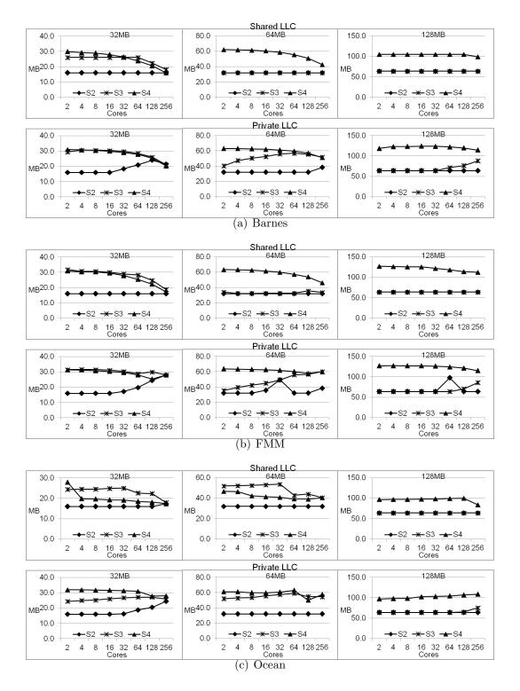
Figure 6.7: Optimal  $LLC_{size}$  at different problem sizes (S2-S4), total cache sizes (32M-128M), and the number of cores for Barnes, FMM, and Ocean.
