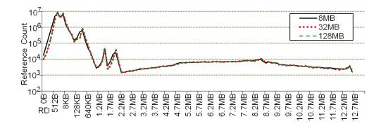
Figure 5.2: CRD profiles from the FFT benchmark running on 64 cores at the S2 problem size across 8M, 32M, and 128M LLC capacity.
