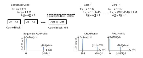
Figure 3.6: A simple example showing how CRD and PRD shift with core count scaling. Each cache block contains 4 elements.
