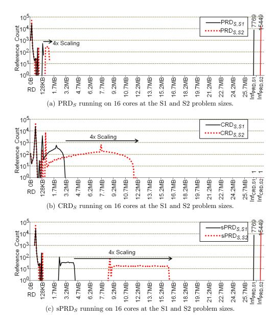
Figure 3.13: FFT's shared-data locality profiles running on 16 cores at the S1 and S2 problem sizes.
