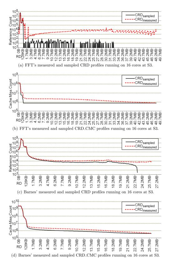
Figure 7.1: Measured and sampled  $CRD_{direct}$  profiles with  $R_{sampling} = 0.1$  and  $R_{pruning} = 0.99$ .
