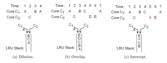
Figure 2.2: Two interleaved memory reference streams, illustrating dilation, overlap, and intercept among inter-thread memory references in the shared cache.
