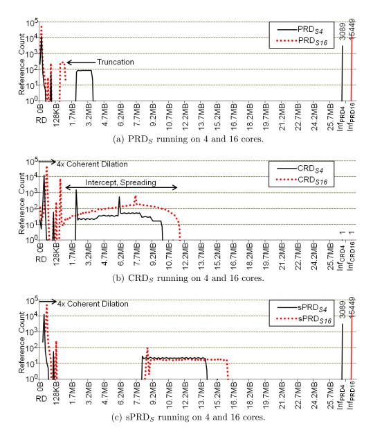
Figure 3.10: FFT's shared-data locality profiles running on 4 cores and 16 cores at the S2 problem size.
