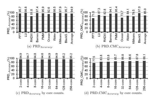
Figure 7.4: Accuracy of the sampling technique with  $R_{Sampling} = 0.1$  and  $R_{Pruning} = 0.99$  for PRD profiles.
