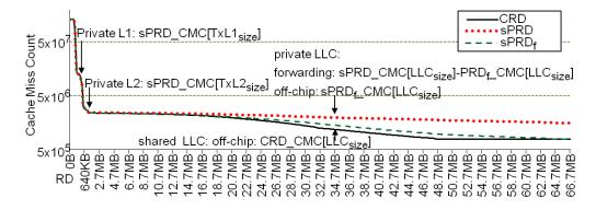
Figure 6.1: CRD\_CMC, sPRD\_CMC, and sPRD<sub>f</sub>\_CMC profiles for FFT running on 16 cores at the S3 problem size.
