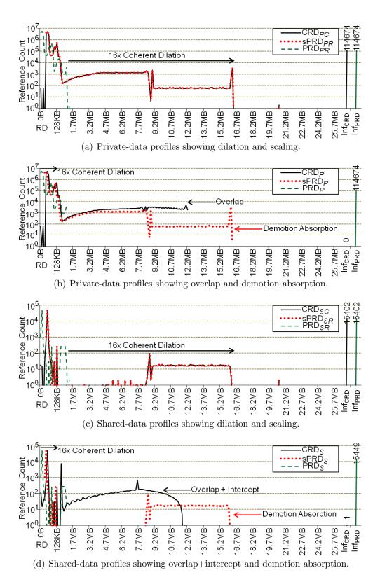
Figure 3.4: FFT's locality profiles for the most important parallel region running on 16 cores at the S2 problem size.
