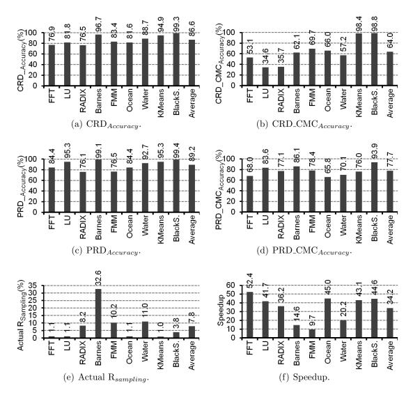
Figure 7.5: Accuracy and performance of the sampling technique with  $R_{Sampling} = 0.01$  and  $R_{Pruning} = 0.90$  for CRD and PRD profiles.
