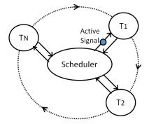
Figure 2.4: Thread interleaving mechanism.
