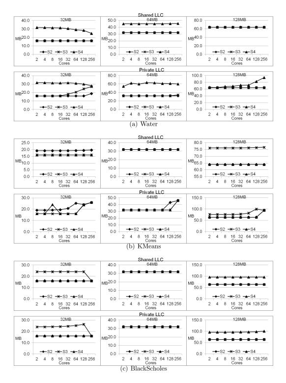
Figure 6.8: Optimal  $LLC_{size}$  at different problem sizes (S2-S4), total cache sizes (32M-128M), and the number of cores for Water, KMeans, and BlackScholes.
