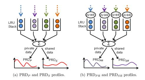
Figure 3.2: Acquiring  $PRD_P$ ,  $PRD_S$ ,  $PRD_{PR}$ , and  $PRD_{SR}$  profiles.
