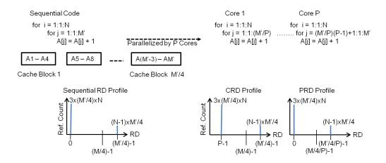
Figure 3.11: A simple example showing how CRD and PRD shift with problem size scaling. Each cache block contains 4 elements.
