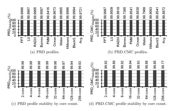
Figure 5.5: Stability measurement of PRD profiles and PRD\_CMC profiles.
