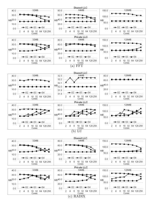
Figure 6.6: Optimal  $LLC_{size}$  at different problem sizes (S2-S4), total cache sizes (32M-128M), and the number of cores for FFT, LU, and RADIX.
