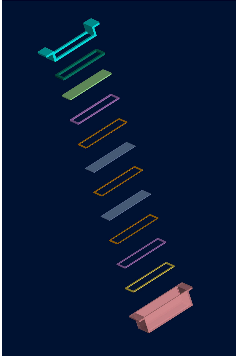
Figure 2.12: Exploded view of the MCP stack as a rough sketch for all the parts. From bottom to top are the outer housing, the grid frame, an insulating ring, electrical contact, the first MCP, electrical contact, second MCP, electrical contact, insulator, the anode board, the spring plate, and the inner housing. Not shown in this sketch are the tabs on the electrical contacts or the ears on the inner housing.
