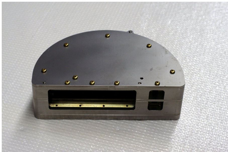
Figure C.7: The completed magnetic circuit. Stainless steel roll pins are used to align the parts. Brass screws secure the clamps to keep the magnets from shifting on launch.
