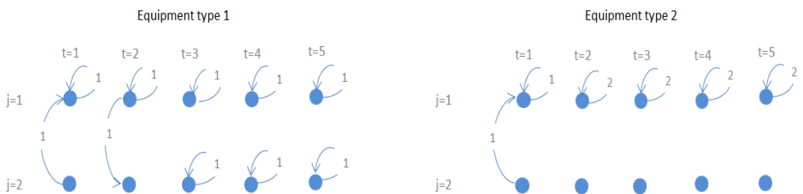
Figure 4.15- Owned equipment fleet deployment plan in example #5 (Numbers shown on arrows are number of shipped pieces of owned equipment)
