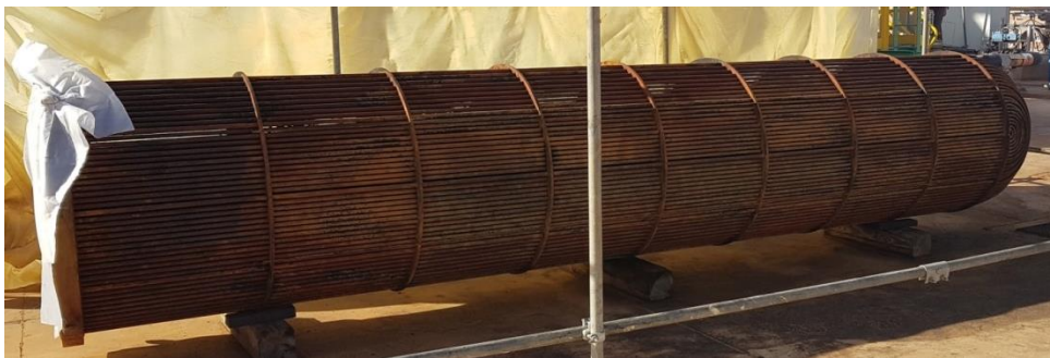
Figure 2. The tube bundle after cleaning
