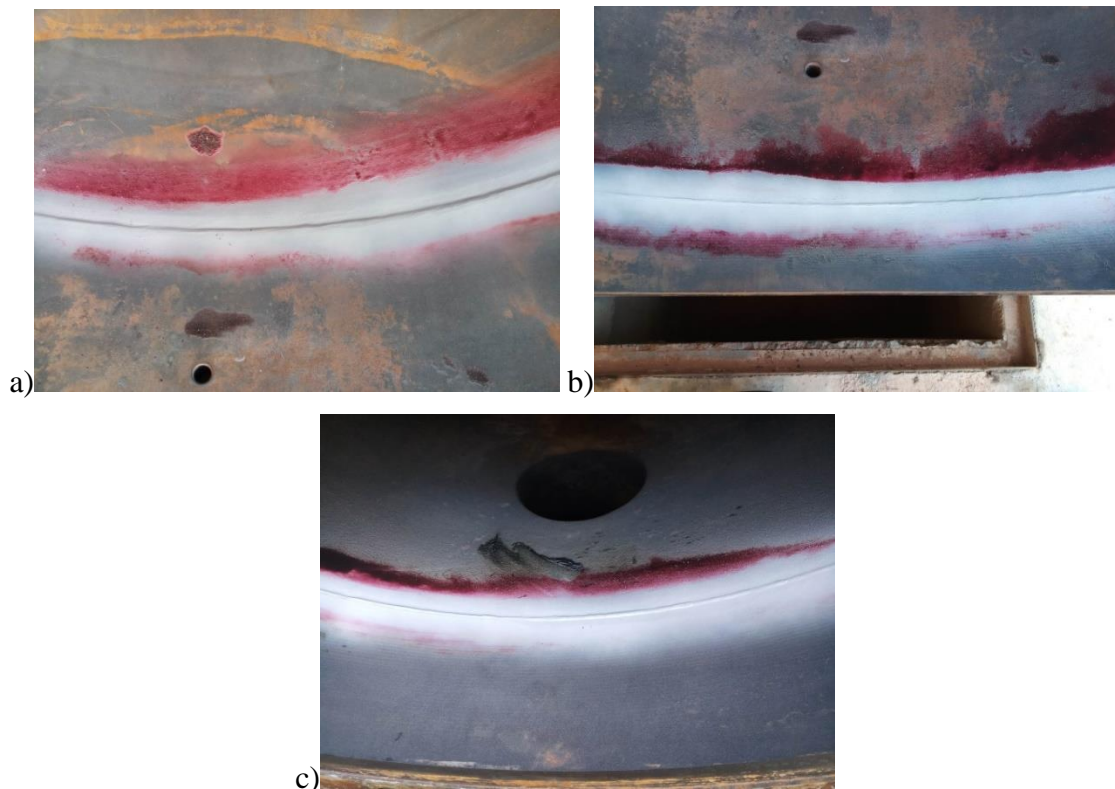
Figure 6. Results of PT tested of the weld joints a) 1 b) 2 and c) 6.
