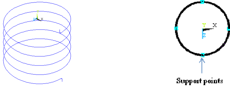
Figure 23: Helical tubes (left) and top view of tubes with support points (right)
