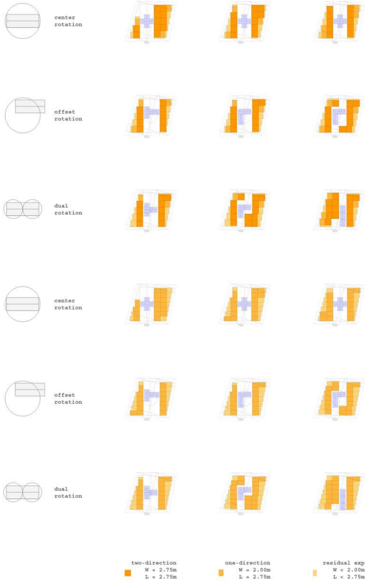
Figure 10-1-2. Versioning of horizontal layout of garage and turntable positioning.
