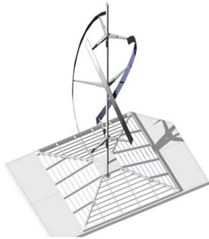
Figure 8-1-4. Vertically elongated wind turbines for capturing interior updraft.
