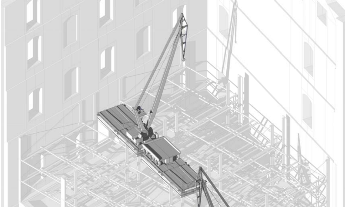
Figure 10-2-2. Construction of scaffolding (primary and secondary structures). The small crane can be moved from turntable to turntable to maximize utility.
