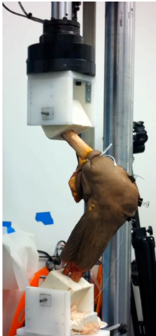
Figure 14. MTS machine fixture. Photograph of a test leg loaded into the MTS machine fixture and attached to the MTS machine at a moment of flexion during the mechanical loading protocol.
