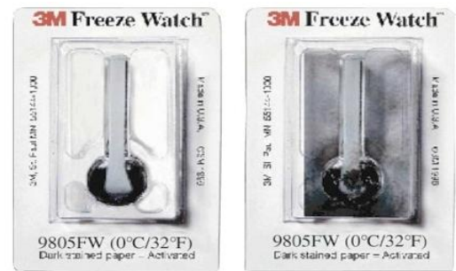
Figure 3: FreezeWatch indicator with instructions for recognizing frozen vaccines Non-Activated Activated When exposed to freezing temperatures, the liquid dye in the monitor freezes, which causes it to fracture and stain the indicator paper. Two Easy Steps 1. Peel off the liner on the back of the indicator. 2. Secure the indicator inside the shipping container or on the product, and interpret results.
