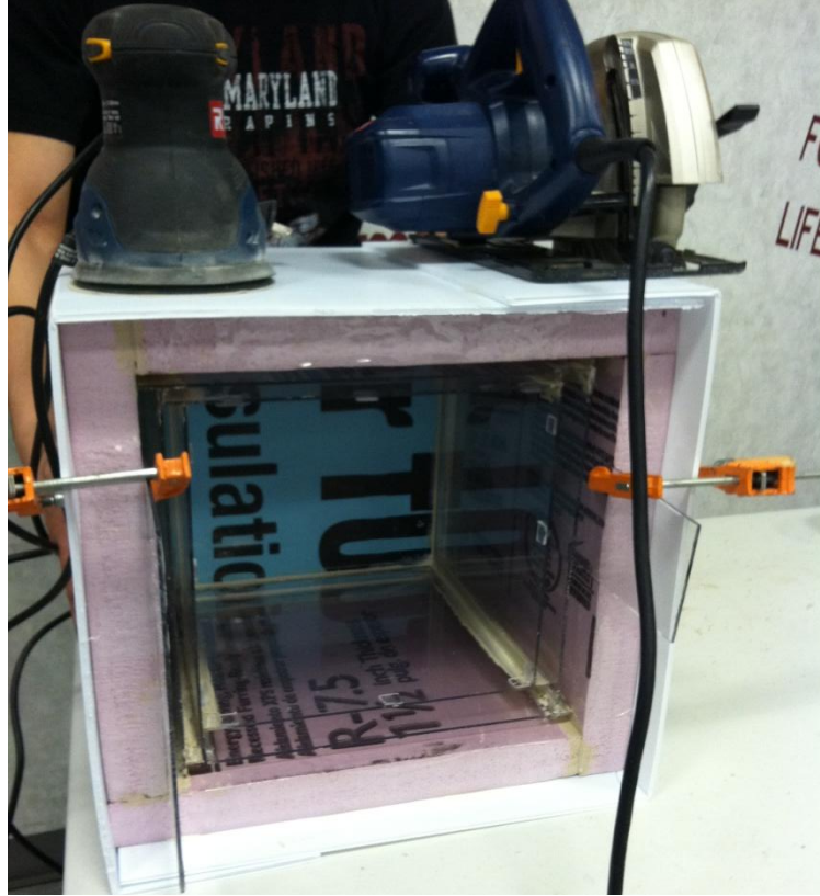
Figure 72: Corrugated plastic (white border) drying around box. Weights (power sander and circular saw) and C-clamps were used to apply pressure while drying.
