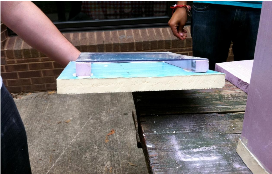
Figure 63: Finished PCM slot on underside of box cover
