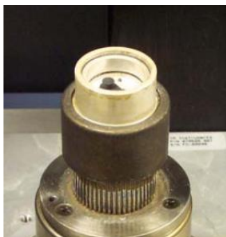
Figure 5: Image of sample containment in q100 series DSC
