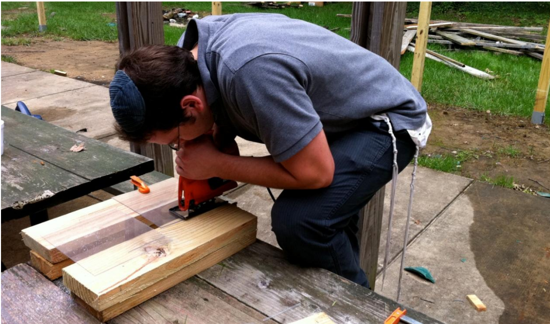
Figure 58: Cutting a sheet of Lexan using the Black and Deck jigsaw
