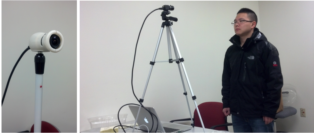
Figure 5.2: The final prototype consists of a digital camera screw mount on a white cane and a plastic shell casing. This mount is easily detachable and can be attached to a camera tripod as well
