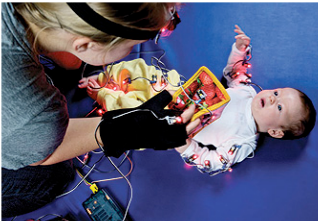
Figure 13: Motion capture suit in use at University of Miami. Note both the tightly-wound cords which could cause discomfort, affecting natural movement and the blinking lights which could distract the infant.
