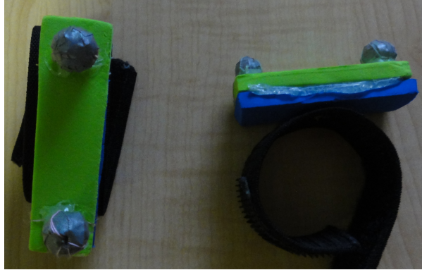
Figure 20: Original Velcro wrist straps. Note the two reflective markers to track position. Foam supports stabilized and elevated reflective markers on wrists.
