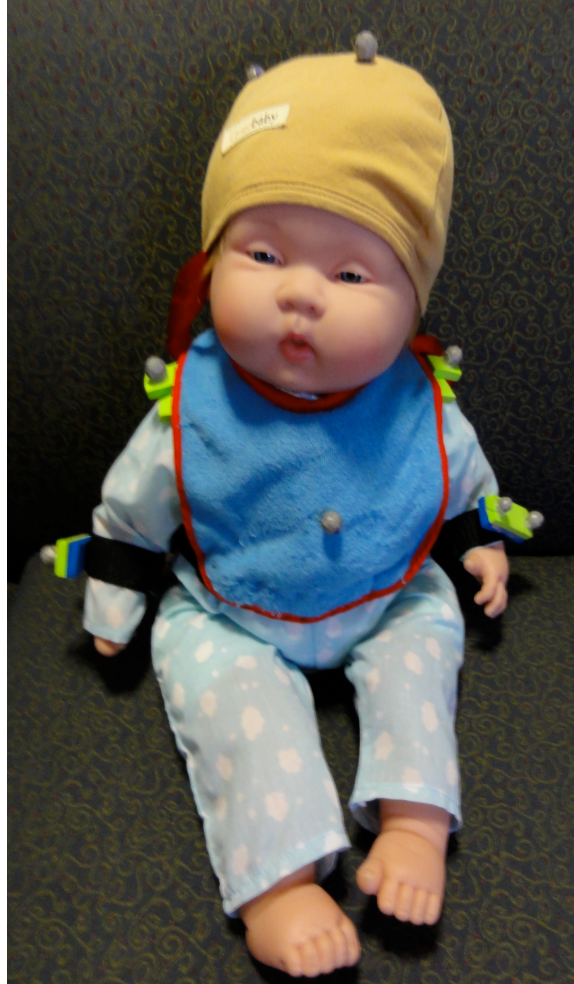
Figure 14: Final suit design. Note the modified commercially-available bib and cap and the original Velcro wrist straps. On the bib, note modifications including fastenable strap, foam supports, and three reflective markers. On the cap note modifications including the chin strap and three (two visible) reflective markers.
