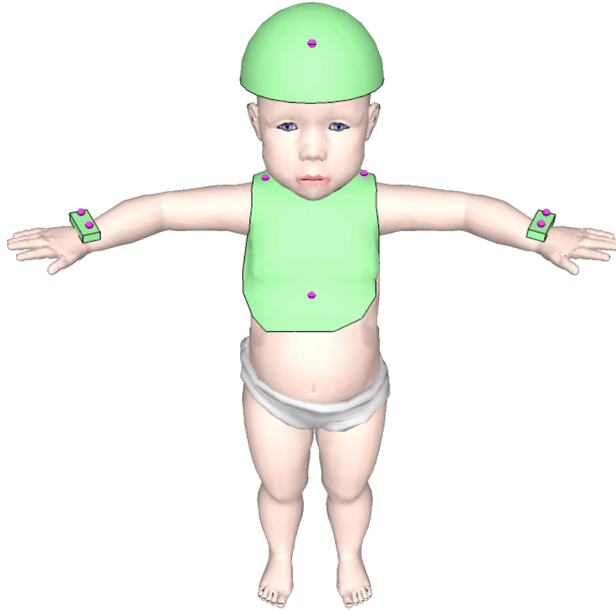
Figure 15: Front view of final infant motion capture suit.
