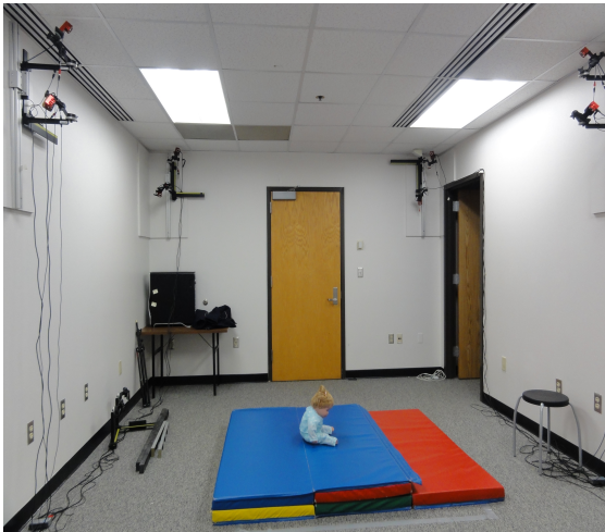
Figure 10: Photograph of lab arrangement. Notice the cameras surrounding and facing the gym mat. The doll represents the approximate location of the capture volume, in which the infant would perform the designated tasks.
