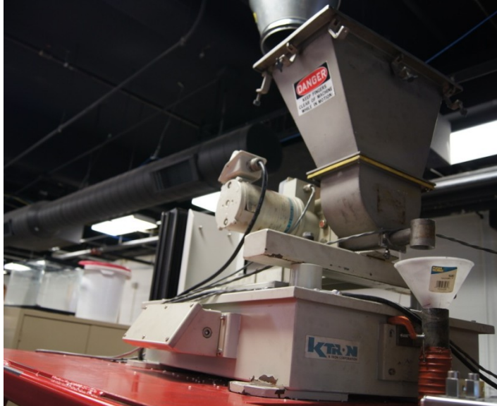
Figure 3.4 - K-TRON loss-in weight pellet feeder
