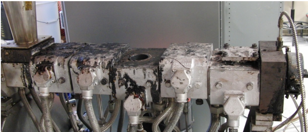
Figure 3.2 - Arrangement of barrels and die zone
