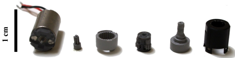
Figure 4.21: Planetary Geared Pager Motor Disassembled
