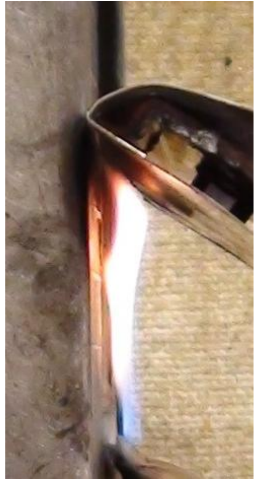
Figure 4. Measured propane burner heat flux profile as a function of time after ignition. A close up image of the propane burner above a sample has been included on the right to help visualize the physical conditions producing this heat flux distribution.
