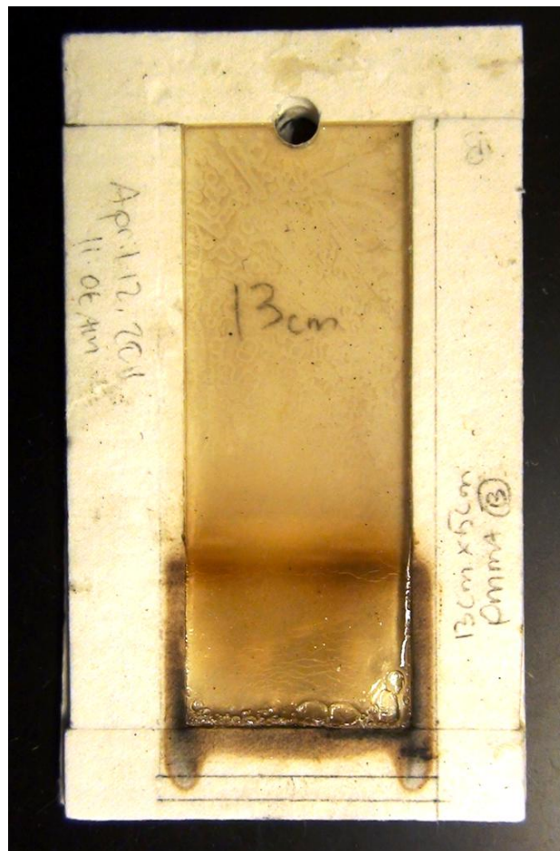
Figure 22. 13 cm sample following burner exposure in a test that did not produce ignition. Note the two regions of elevated pyrolysis- one directly at the sample's base and the second, smaller region, at 3.5 cm (closest to the burner shield)
