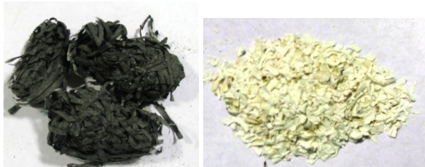
Figure IV-11. Char leftover from pyrolysis (left) and ash leftover from gasification (right)
