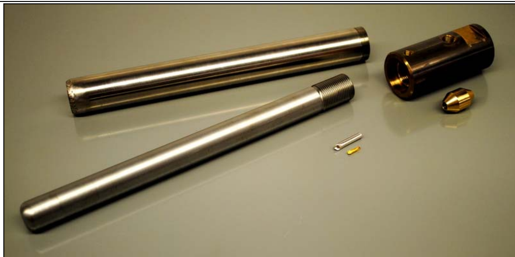
Figure 3-9 (middle) For hydrothermal experiments, an inner capsule of Au or Cu–Au alloy was placed inside a platinum capsule (30 mm length in picture). The combined capsule was placed inside a TZM or MHC (lower grey tube in picture) pressure vessel which was placed within an Inconel alloy sheath (top tube) which was flushed with argon to prevent oxidation of the pressure vessel. Water cooling kept the Al–Ni Bronze fitting and Cu–Al connector at \sim 20^{\circ}\text{C} for a rapid quench.
