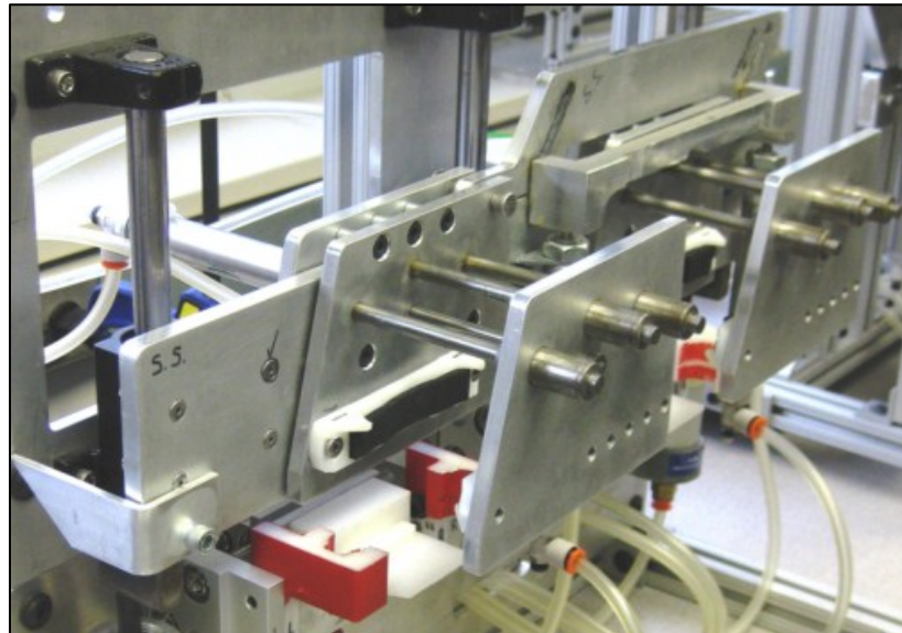
Figure 6.4 Filament Jaw Assembly (Shown as Fabricated).
