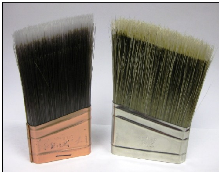
Figure 6.6 Knot Samples Tested: (Left) 2" Knot with Silver Tip Nylon Synthetic Filaments; (Right) 2.5" Knot with Nylon and White Pig Hair Natural Filament Blend.
