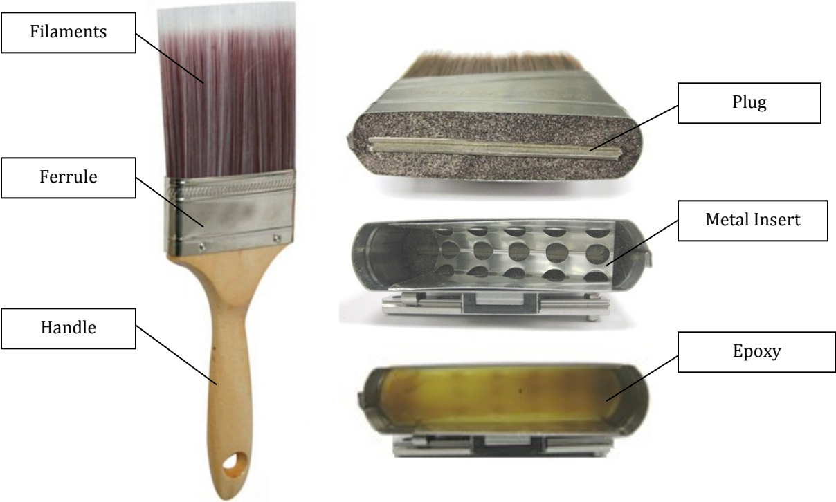
Figure 1.1 Paint-Brush Components.
