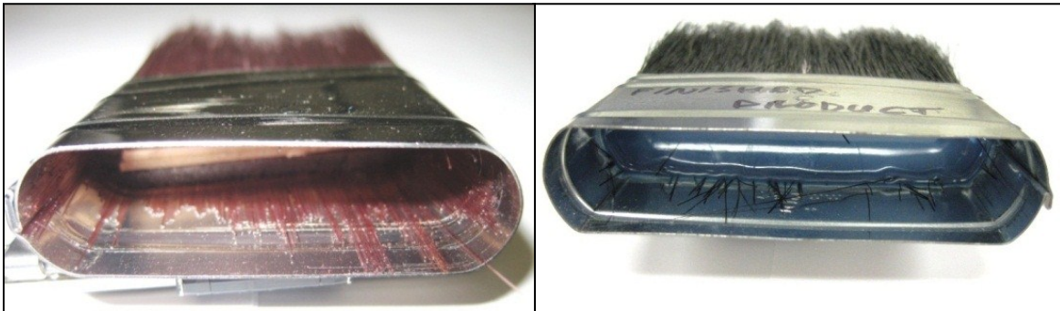
Figure 1.9 (Left) Dragback after Insertion of the Gauging Block; (Right) Dragback after Epoxy Filling and Curing.
