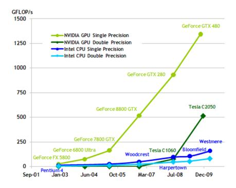
Figure 2.1: [color] Growth in the CPU and GPU speeds over the last 6 years on benchmarks (Image from [63])
