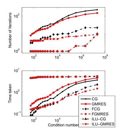
Figure 4.4: [color] Performance of the proposed preconditioner with CG and GMRES against ILU-preconditioned and unpreconditioned versions
