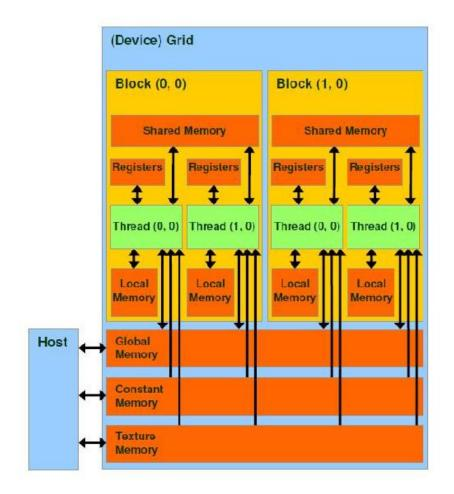
Figure 2.2: [color] Logical organization of the GPU memories as seen through CUDA (Image from [63])
