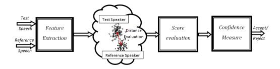
Figure 6.1: [color] A modular representation of a generic speaker recognition system
