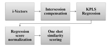
Figure 8.3: One-shot schematic for speaker recognition.
