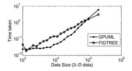
Figure 2.4: Performance of GPUML for Gaussian kernel summation compared to FIGTREE[58], the linear algorithm for various data sizes at 3-dimensions dimensions.
