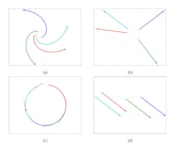
Figure 2.4: These figures illustrate the planar trajectories which correspond to the four types of pure shape equilibria, including spirals (figure 2.4a), expansion/contraction without rotation (figure 2.4b), circling equilibria (figure 2.4c), and rectilinear equilibria (figure 2.4d).
