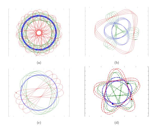
Figure 3.7: These MATLAB plots illustrate 3-particle motions in the plane for different initial conditions arising in the  $\alpha = \pi/2$  case. The associated phase space i.e.  $(\phi, \tilde{\lambda})$  trajectories are periodic, and result in the precessing behavior in physical space depicted here.
