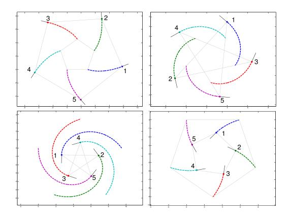
Figure 2.6: This figure illustrates the four unique pure shape equilibria which exist for the particular case  $\alpha_1 = \alpha_2 = \alpha_3 = \alpha_4 = \alpha_5 = \pi/2$ . In each figure, initial conditions were chosen such that the particle formation started in one of the pure shape equilibrium configurations.
