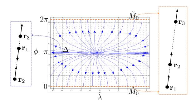
Figure 3.4: Depiction of the  $\{\phi, \tilde{\lambda}\}$  phase portrait for the  $\alpha = 0$  case, which should be viewed as a (punctured) cylinder which has been cut along the set  $\tilde{M}_0$ and unwrapped. Also depicted are representative particle formations (from the full physical space) which correspond to each of the invariant submanifolds  $\tilde{M}_0$  and  $\Delta$ .
